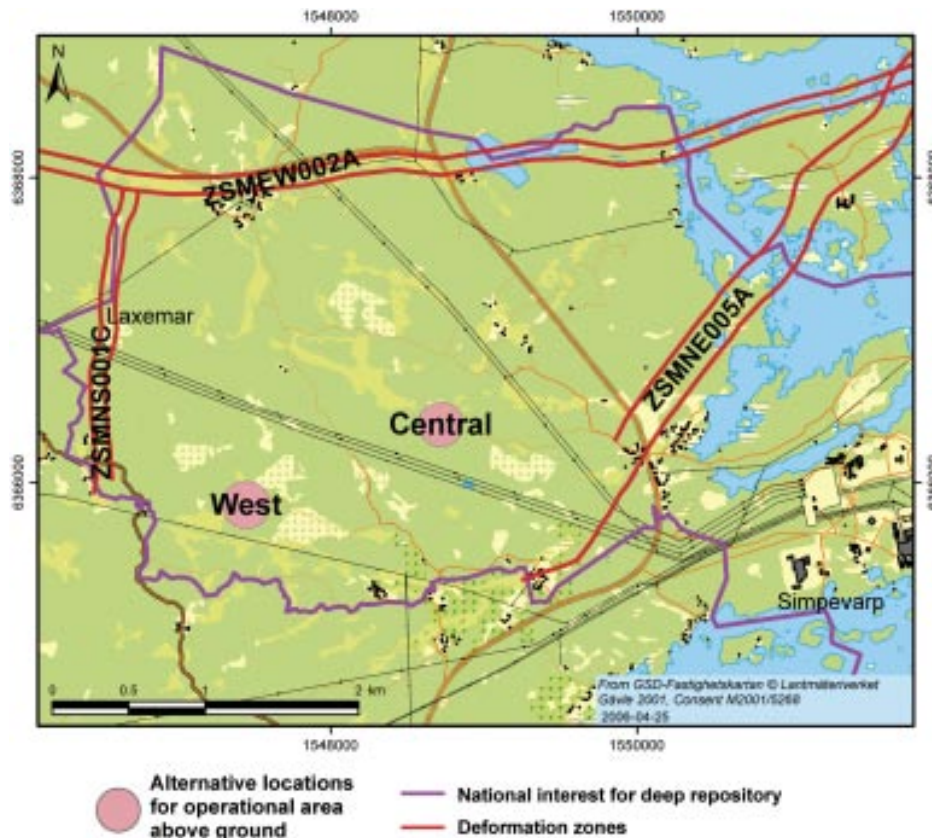
Figure 5-1. Alternative locations for an operational area above ground designated Central and West. The figure also shows how the Laxemar area is delimited by deformation zones and national interest for a deep repository.
