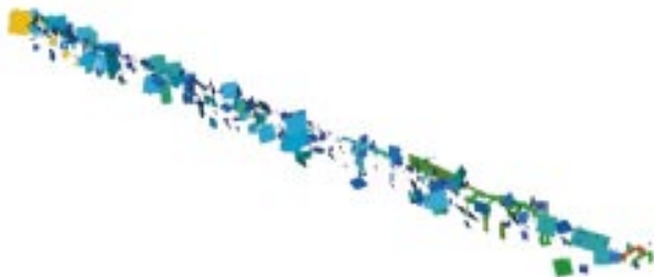
Figure 4-17. An example of a number of joints that intersect the 38 deposition holes from an NAPSAC generation.
