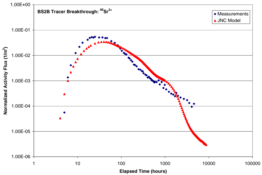
Figure 7-10: Step 2 CN Model, Structure 19 Pathways (Path I), ^{85}\text{Sr}^{2+} , tracer injection in KI0025F02_R3.
