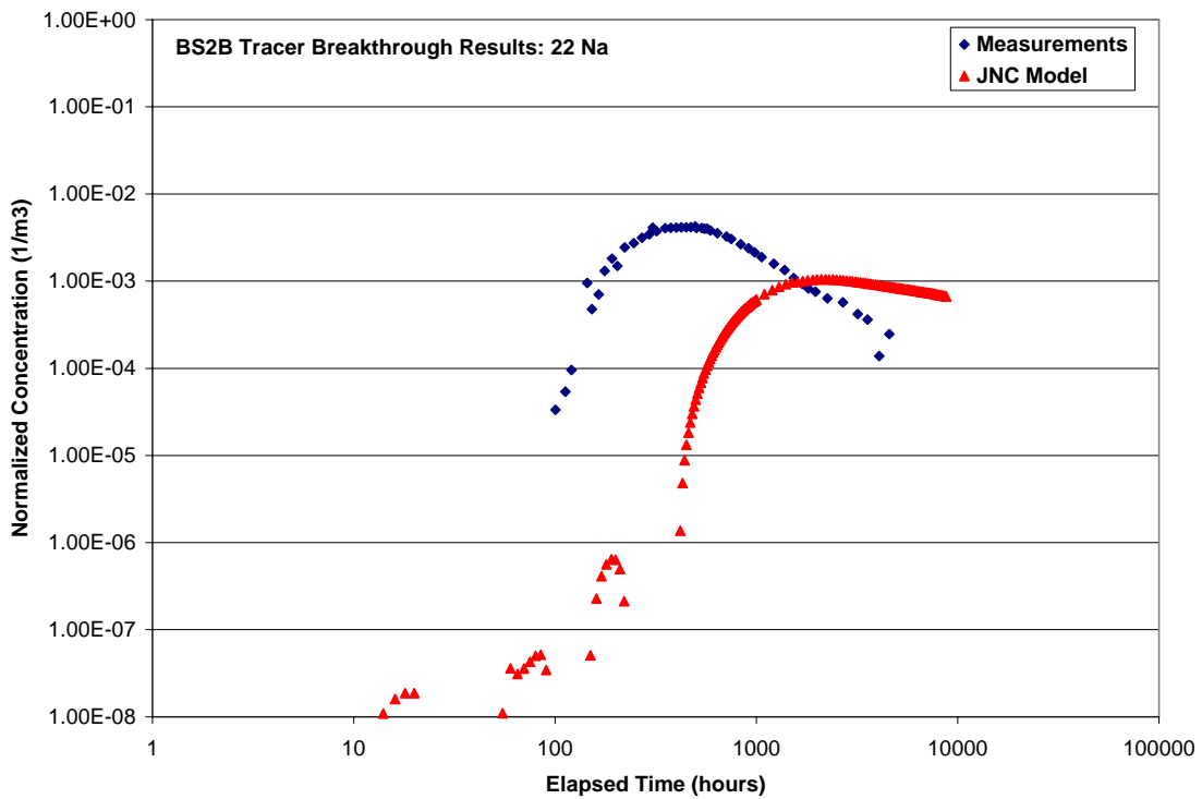
Figure 7-23: Breakthrough curve for ^{22}\text{Na}^+ , Path II (BG1), stochastic background fracture model MC5.
