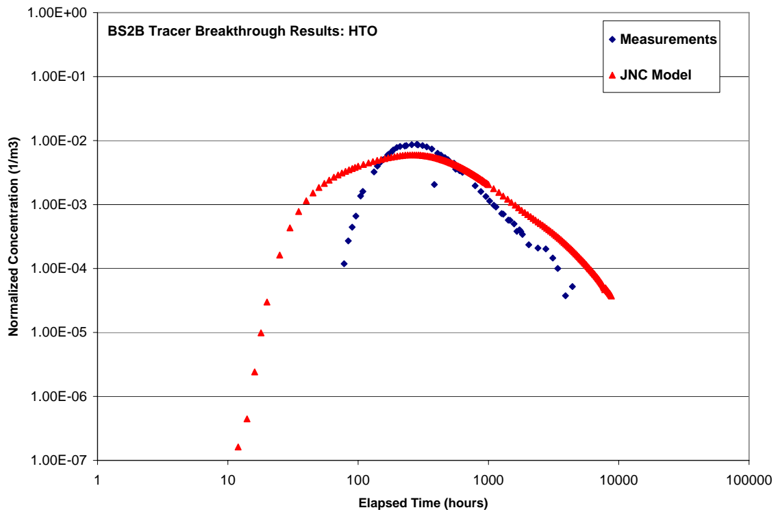
Figure 7-21: Breakthrough curve for HTO, Path II (BG1), stochastic background fracture model MC5.
