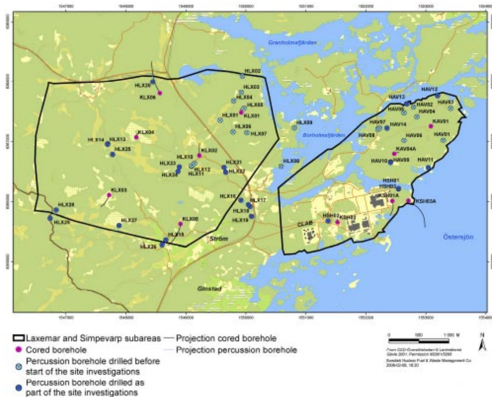
Figure 1-6. Overview map of the locations of core-drilled and percussion-drilled boreholes in the Laxemar (on the left hand side) and Simpevarp (on the right hand side) subareas.
