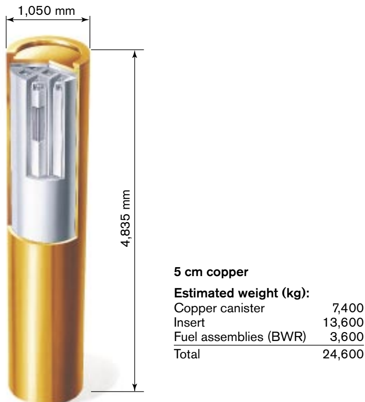
Figure 1-4. Weights and dimensions for the canister for disposal of BWR fuel.
