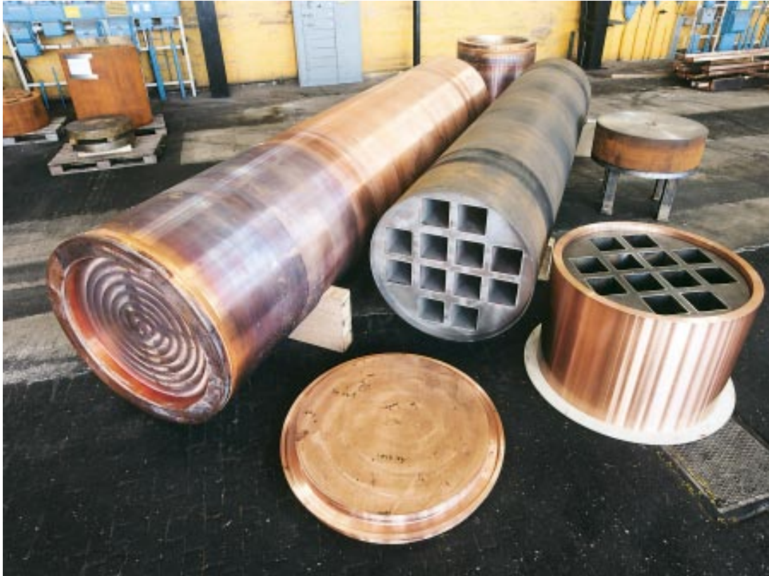
Figure 4-2. Canisters parts, cast iron insert, copper tube and lid. A short section of a canister with insert is also shown.
