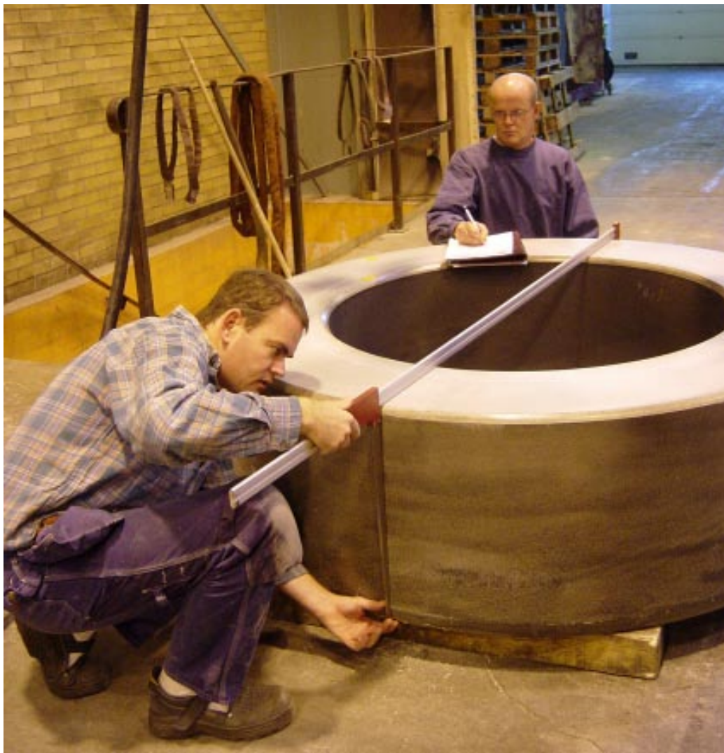
Figure 5-1. Control measurement of bentonite ring.
