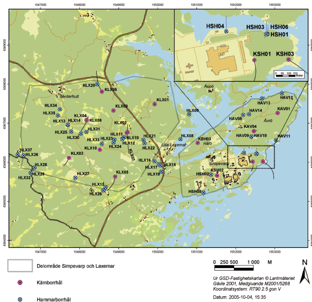
Figure 1-1. Location of all telescopic boreholes drilled up to December 2005 within or close to the Oskarshamn candidate area. The projection of each borehole on the horizontal plane at top of casing is also shown in the figure.
