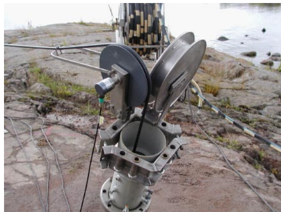
Photo 4. Depth measuring wheel on TOC.
