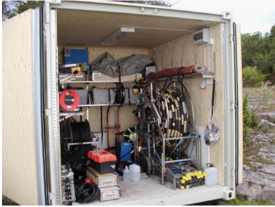
Photo 1. Container with spool for hose.
