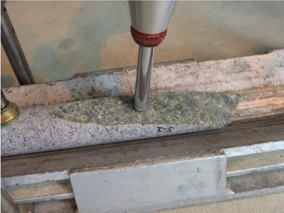
Figure 3-2. Clamp for the Schmidt hammer tests.
