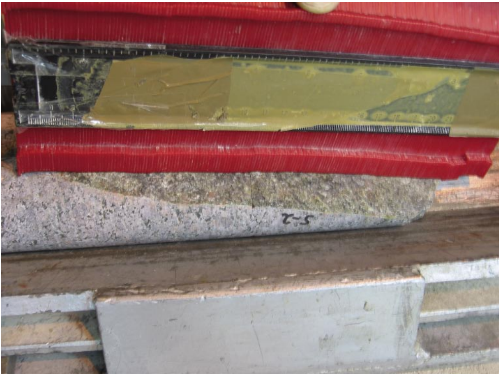
Figure 3-3. Profilometer applied on a joint surface.
