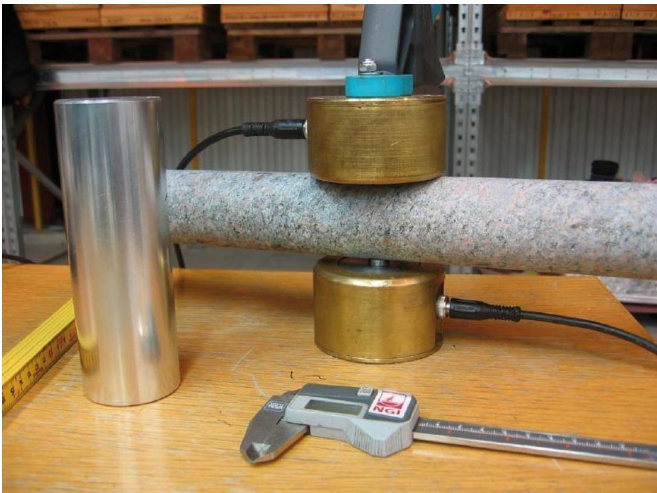
Figure 3-1. Detail of NGI's apparatus for measuring acoustic P-wave travel time transverse on a foliated borehole core. The aluminium cylinder for calibration of the device is on the left.
