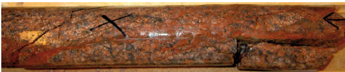
Figure 5-47. Laumontite sealed fracture network. The diameter of the drill core is c 5 cm. KFM01B 434.33–434.70 m.
