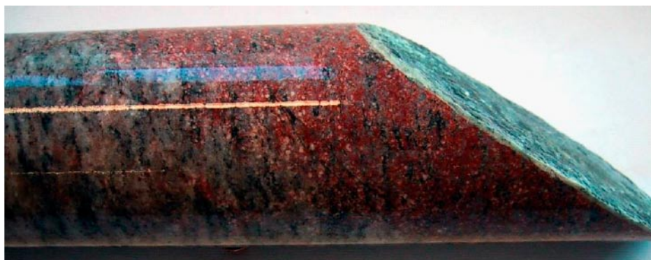
Figure 1-1. Red-coloured altered wall rock adjacent to calcite- and chlorite-coated fracture. The diameter of the drill-core is ~ 5 cm, KFM08A 623.03–623.35 m.
