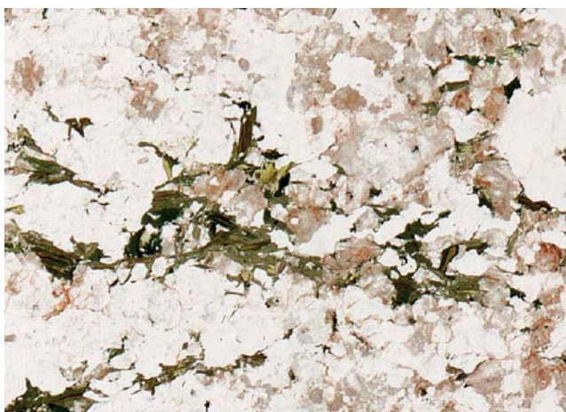
Figure 5-44. Scanned thin section with connected chlorite grains. The base of the figure is \sim 1.5 cm, KFM02A 506.80 m.
