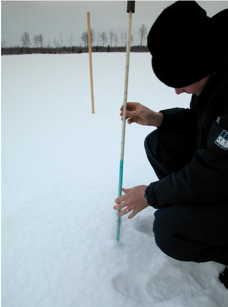
Figure 3-2. Measurement tube for determination of ground frost depth.
