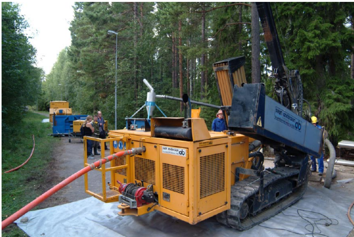
Figure 3-1. The Nemek 407 percussion drilling machine employed for drilling the percussion borehole HFM23 at drill site DS9.
