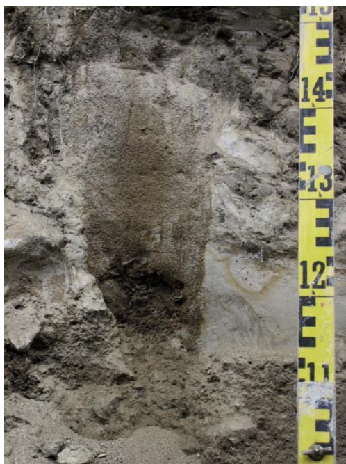
Figure 5-13. At Profile 4 Sliding has partly disturbed the primary stratigraphy and it was therefore difficult to define the different layers. The photo shows post-glacial sand (in the centre), which has been mixed with glacial clay and silt. The profile is situated close to a slope.
