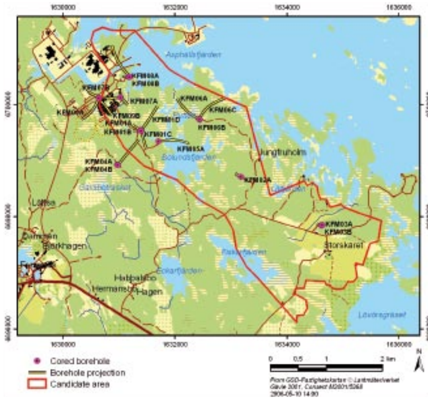
Figure 1-1. The investigation area at Forsmark (approximately the area inside the black square) including the candidate area selected for more detailed investigations with the currently completed core drilled boreholes.
