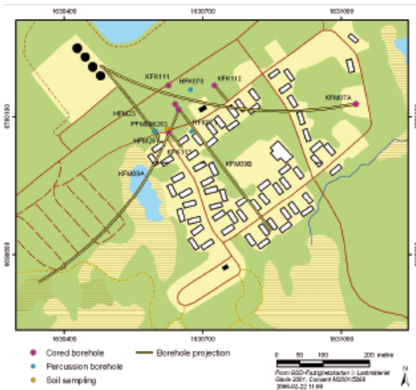
Figure 1-2. Locations and projections on the horizontal plane of the cored boreholes KFM09 and surrounding boreholes at drill sites DS9 and DS7.
