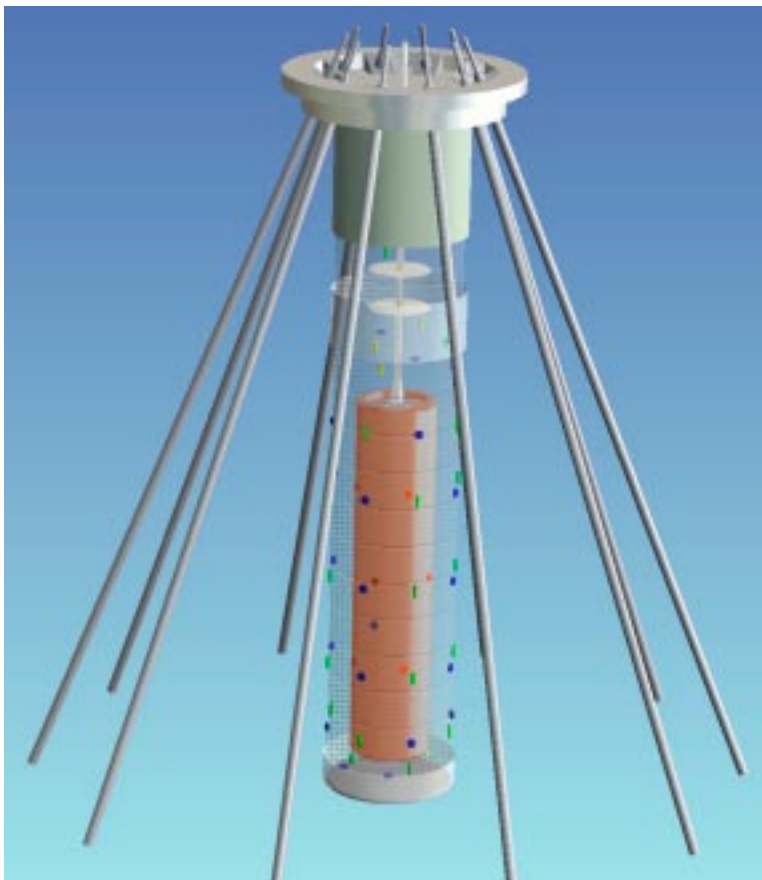
Figure 2-24. Layout of the Lasgit experiment showing the copper canister, the bentonite buffer, the location of some of the instrumentation, the plug and rock anchors.
