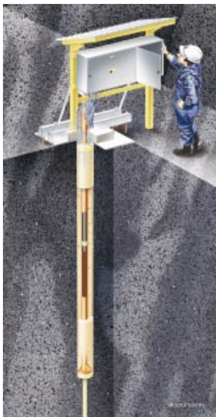
Figure 2-19. Illustration of the experimental set-up in the Long Term Test of Buffer Material (left) and a cross-section view of one S-type parcel (right). In the gauges column, the first figure represents the block number; second figure represents the number of sensors and T, P, W, M indicate temperature, total pressure, water pressure and moisture sensors, respectively.
