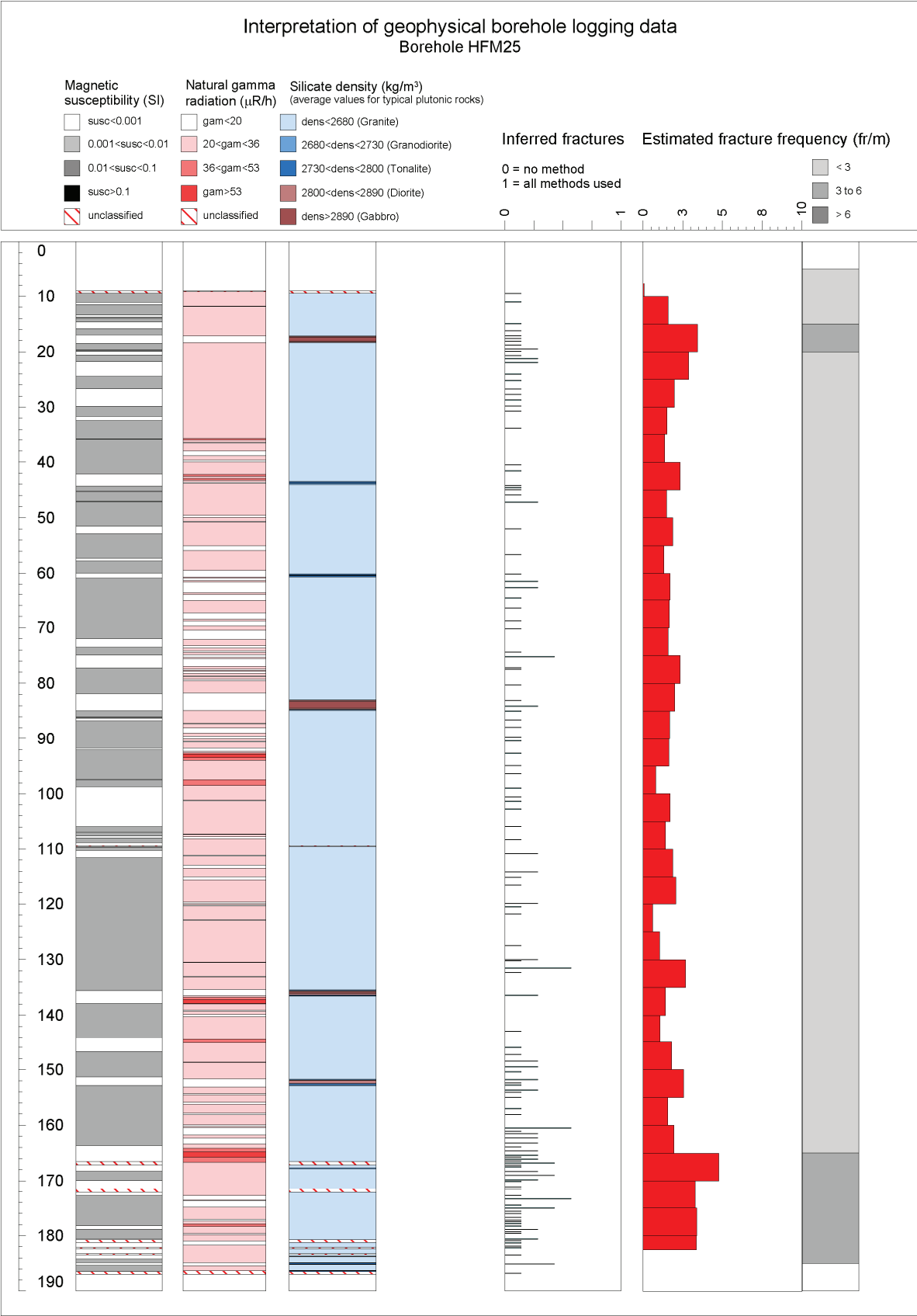
Figure 5-7. Generalized geophysical logs of HFM25.
