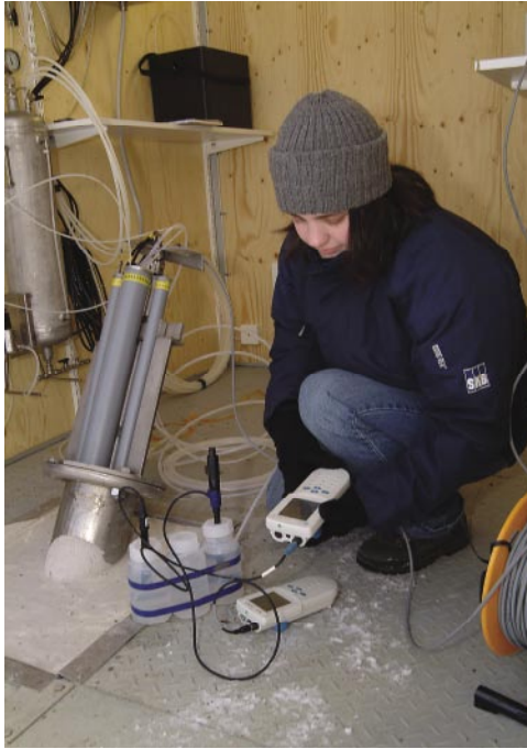
Figure 4-1. Water from the borehole is lead through a measurement cell (consisting of three plastic bottles) to perform field measurements of pH, temperature and conductivity.
