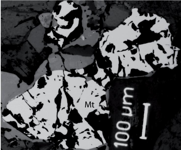
Figure 7-17. Microphotograph of magnetite (Mt) from sample 320G, reflective light.
