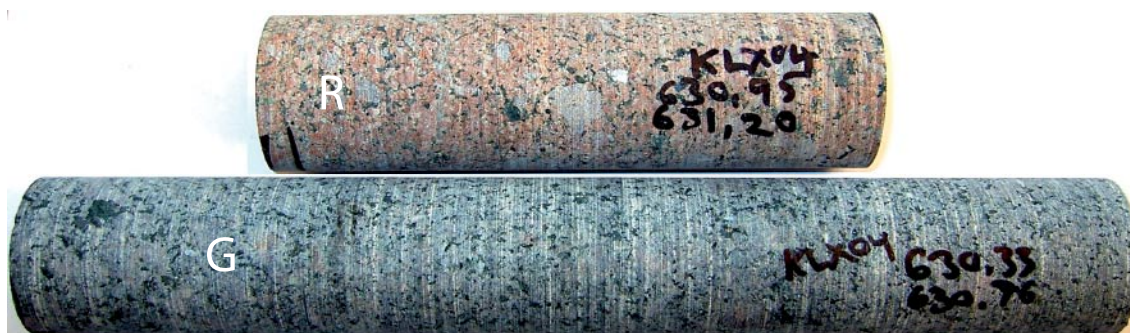
Figure 6-1. Photo of drill core samples 630R (“R”= red-stained rock) and 630G (“G”= reference rock) after they were sawed clean from fractures. Drill core diameter is about 50 mm.
