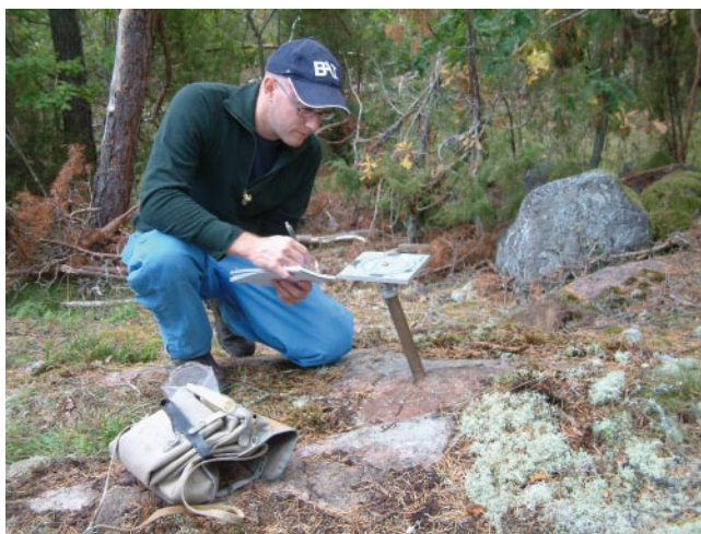
Figure 5-1. a) Petrophysical sampling by use of water cooled drill machine. b) Orientation of drill core by use of sun compass.
