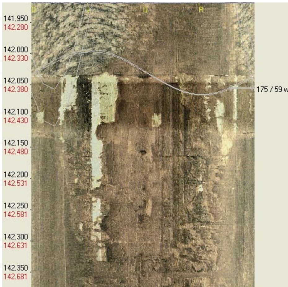
Figure 3-1. Abrupt appearance of a coating on the borehole wall, KFM07B.
