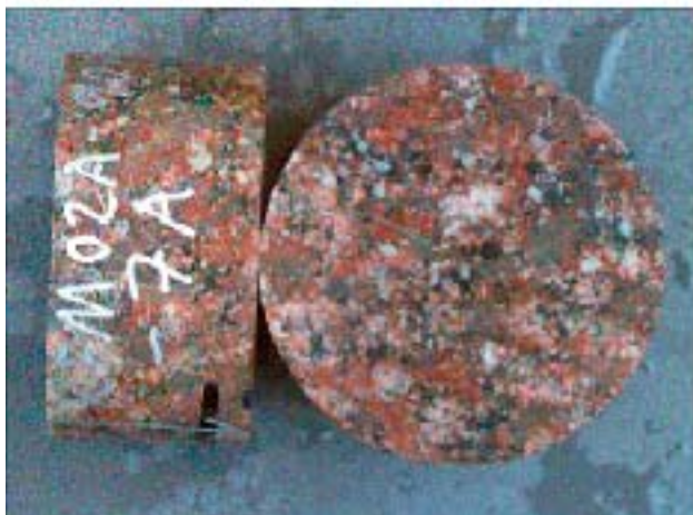
Figure 2-32. Core sample of granite to granodiorite from KFM02A (secup: 528 m) used for measuring thermal properties using the TPS method /Adl-Zarrabi 2004a/. Note the red colouration indicative of oxidation.
