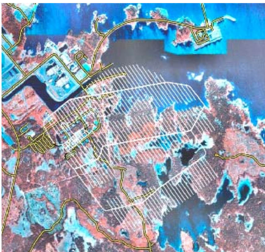
Figure 2. Preliminary layout (February 2005) for a repository at 400 m depth at Forsmark.
