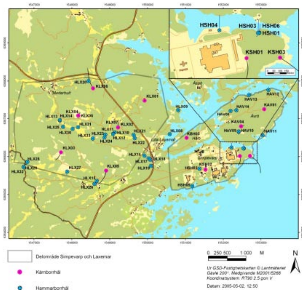
Figure 3-2. The groundwater sampling locations in the Simpevarp area. Location of hydrogeochemically prioritised boreholes KLX01, KLX02, KLX03, KLX04 and KLX06 (Laxemar subarea) and KAV01, KAV04A, KSH01A, KSH02 and KSH03 (Simpevarp subarea). Also indicated are the percussion boreholes, many of which are included in the Laxemar v. 1.2 evaluation.
