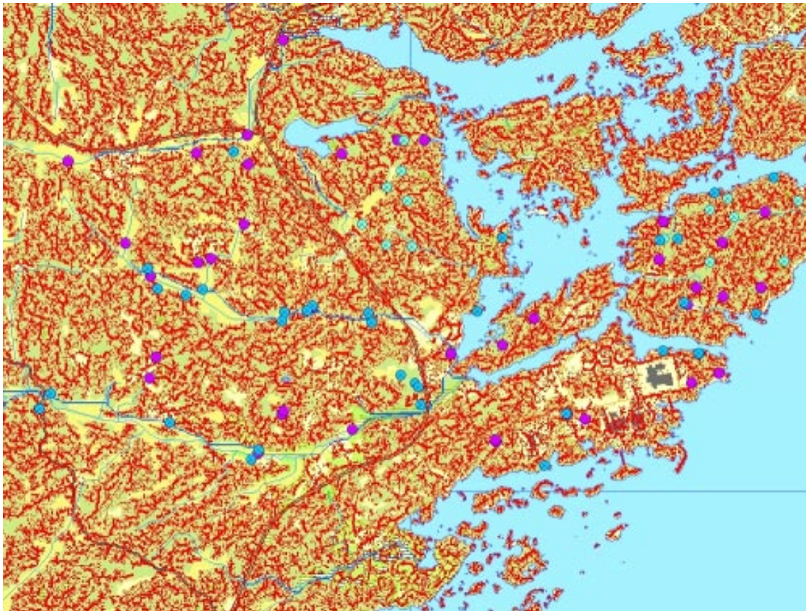
Figure 9-5. Simpevarp area: Topographic/hydrologic-based map showing areas of potential discharge (in blue) and the location of soil pipes (purple infilled circles) and percussion boreholes (blue infilled circles). Green and yellow colouration represent intermediate areas where recharge and discharge can not be satisfactorily distinguished.
