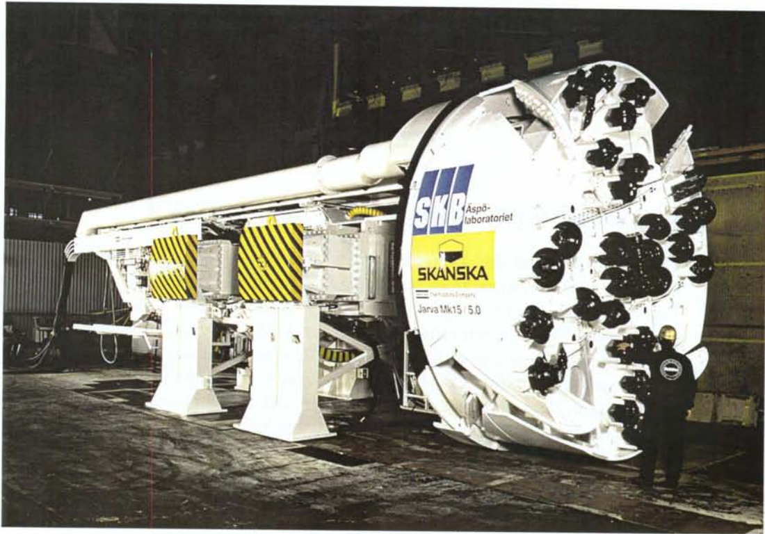
Figure 8-1. The TBM machine used was a 5 m diameter ATLAS COPCO JARVA MK15.
