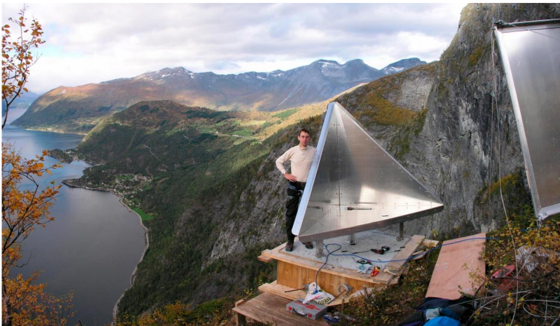
Figure 4-1. Artificial corner reflector installed near Tafjord, in Norway. The reflector is constructed of 10mm thick aluminum.
