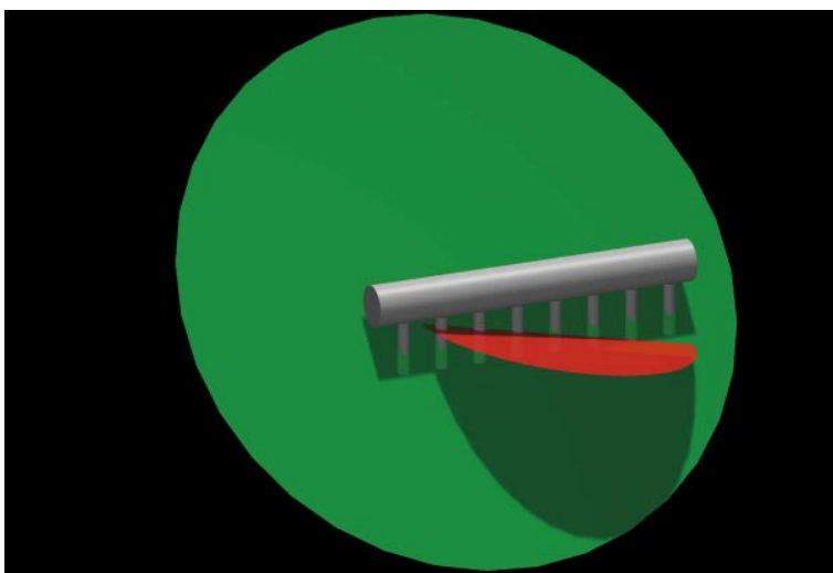
Figure 5-2. A potentially discriminating fracture can remain undetected despite the use of the full perimeter criterion in the deposition tunnel.
