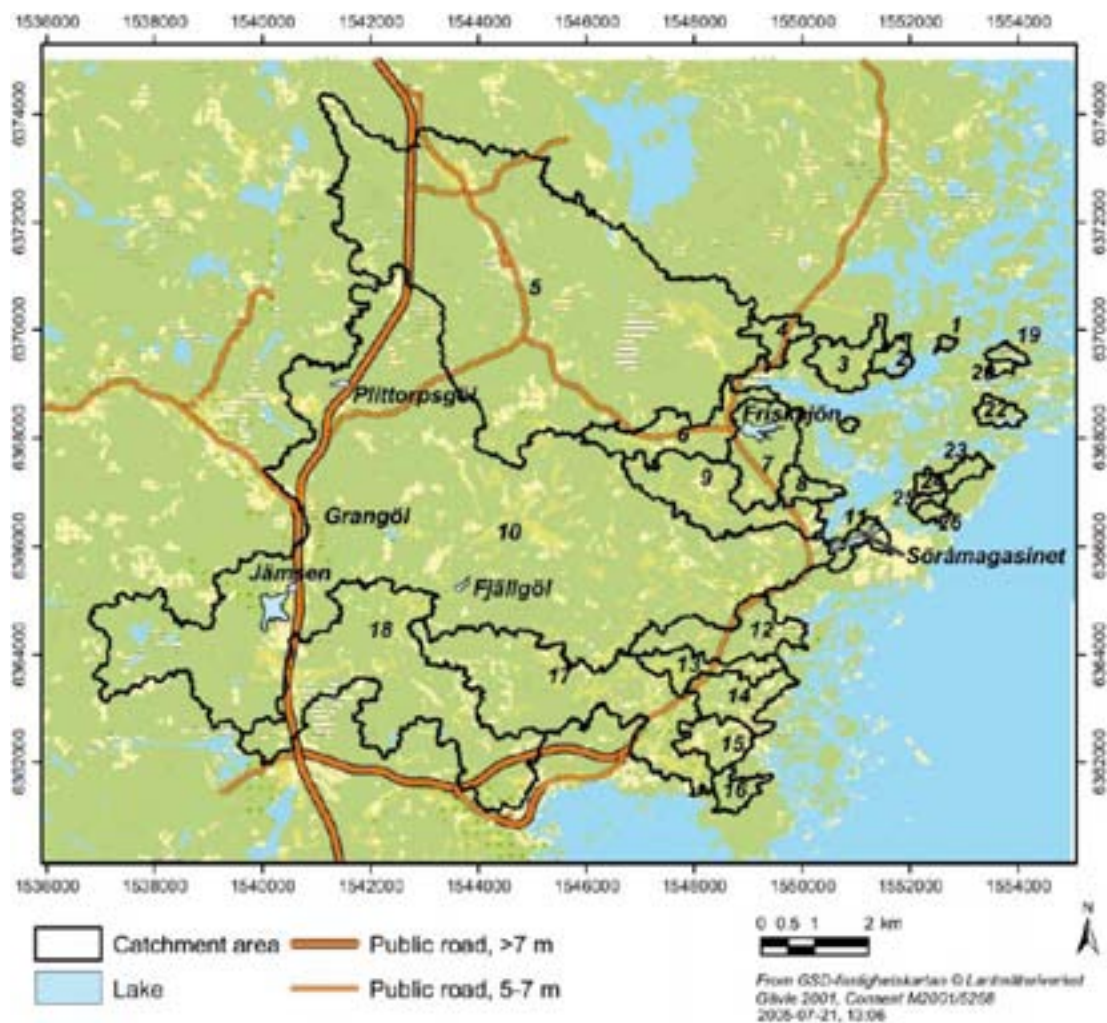
Figure 3-30. Delineation and numbering of the 26 catchment areas in the Simpevarp regional area /Brunberg et al. 2004/. The map also shows the locations of the 6 lakes in the area.
