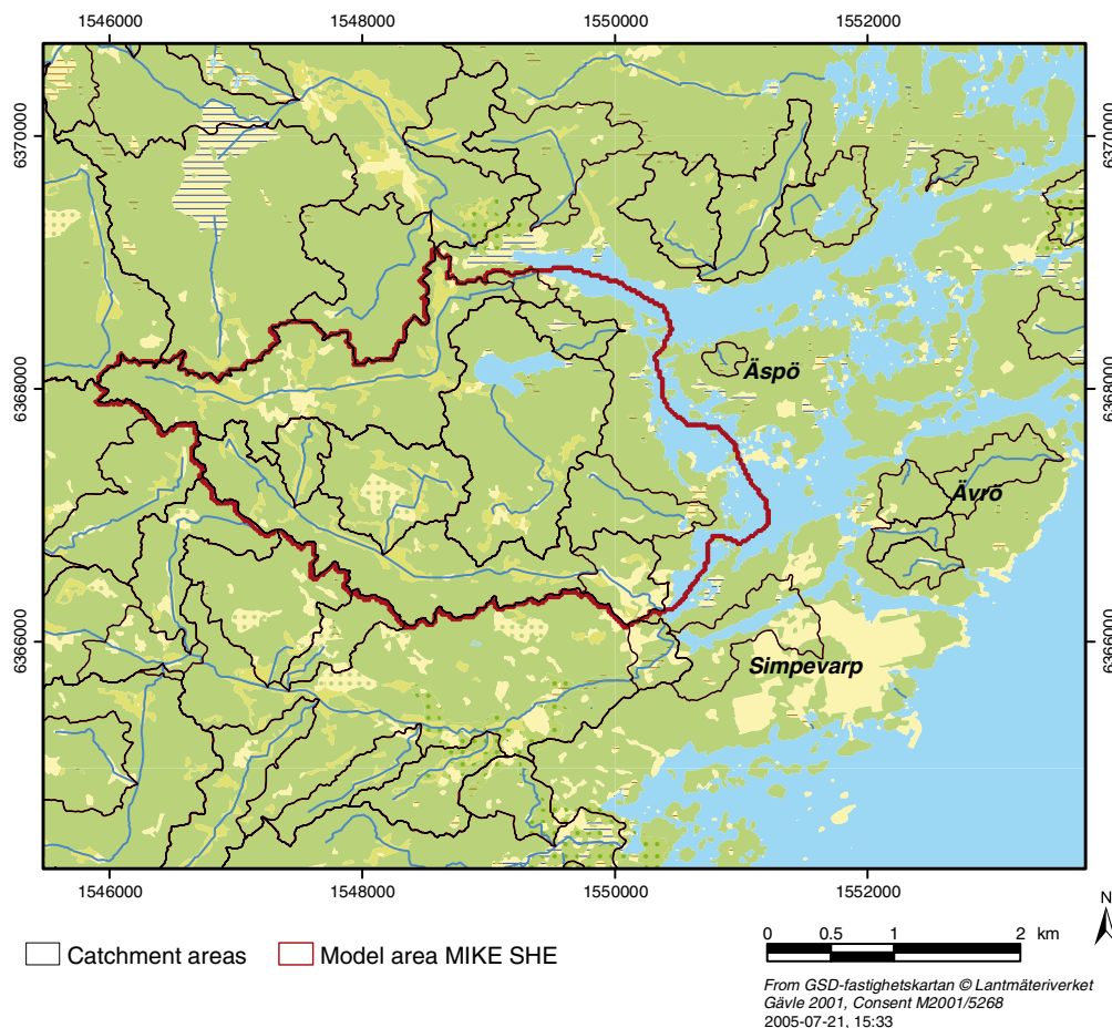
Figure 3-36. Map showing the catchment area boundaries (black lines), and the boundaries of the MIKE SHE-MIKE 11 model area (red line). Note that the model area includes land areas close to the sea, outside (downstream) of catchment areas 6–9, cf /Brunberg et al. 2004/.
