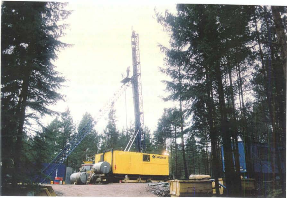
Figure 6.1 The wire-line rig at place showing the rig-floor shelter, the mast and the supporting legs. Notice the man on the derrick platform. Photo K-E Almén.
