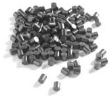
Fuel pellets before they have been used in nuclear power plants. Each pellet has a diameter of one centimetre.
