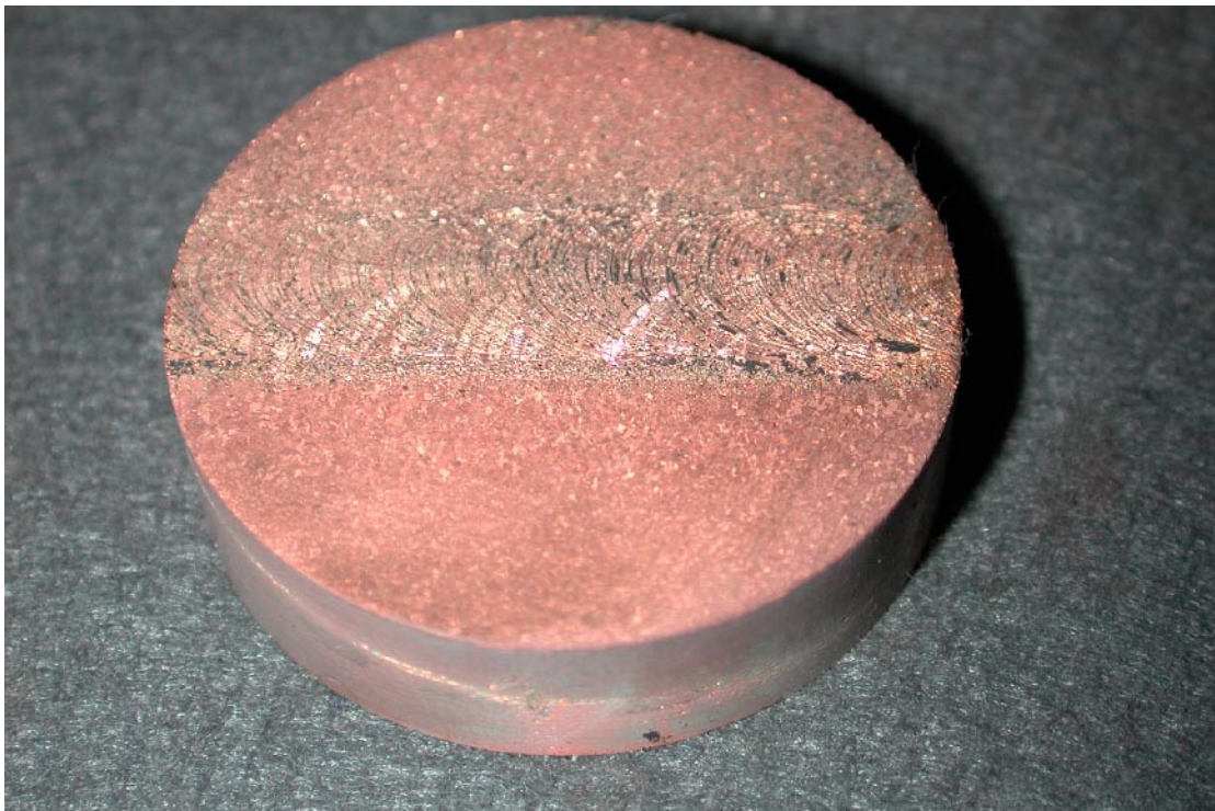
Figure 3-14. Photograph sample L013 after exposure. The grain structure is revealed along weld and markings from the welding process have been etched out of the surface.
