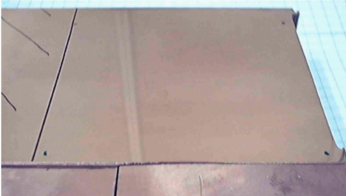
Figure 3-10. Photograph of the sample “Corrosion KL059-COR1/T”. The white lines indicate the SKP scanning area shown in Figure 3-9.
