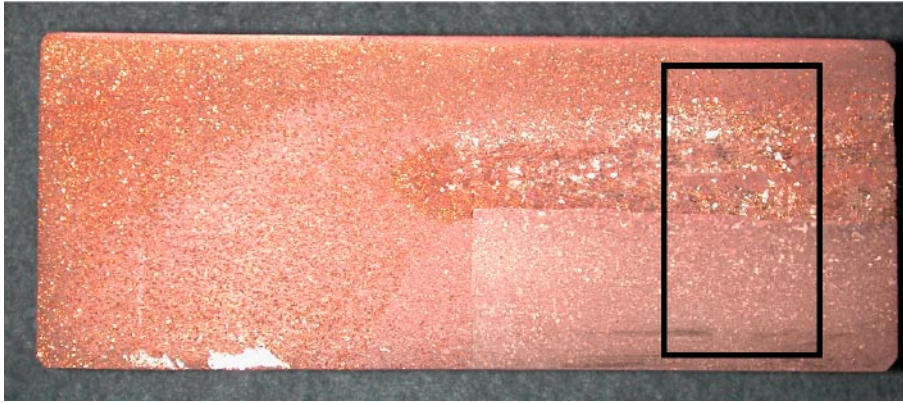
Figure 3-6. Exposed sample revealing canister material and lid material. The marking indicates the scan area of the SKP image above, rotated 90°.
