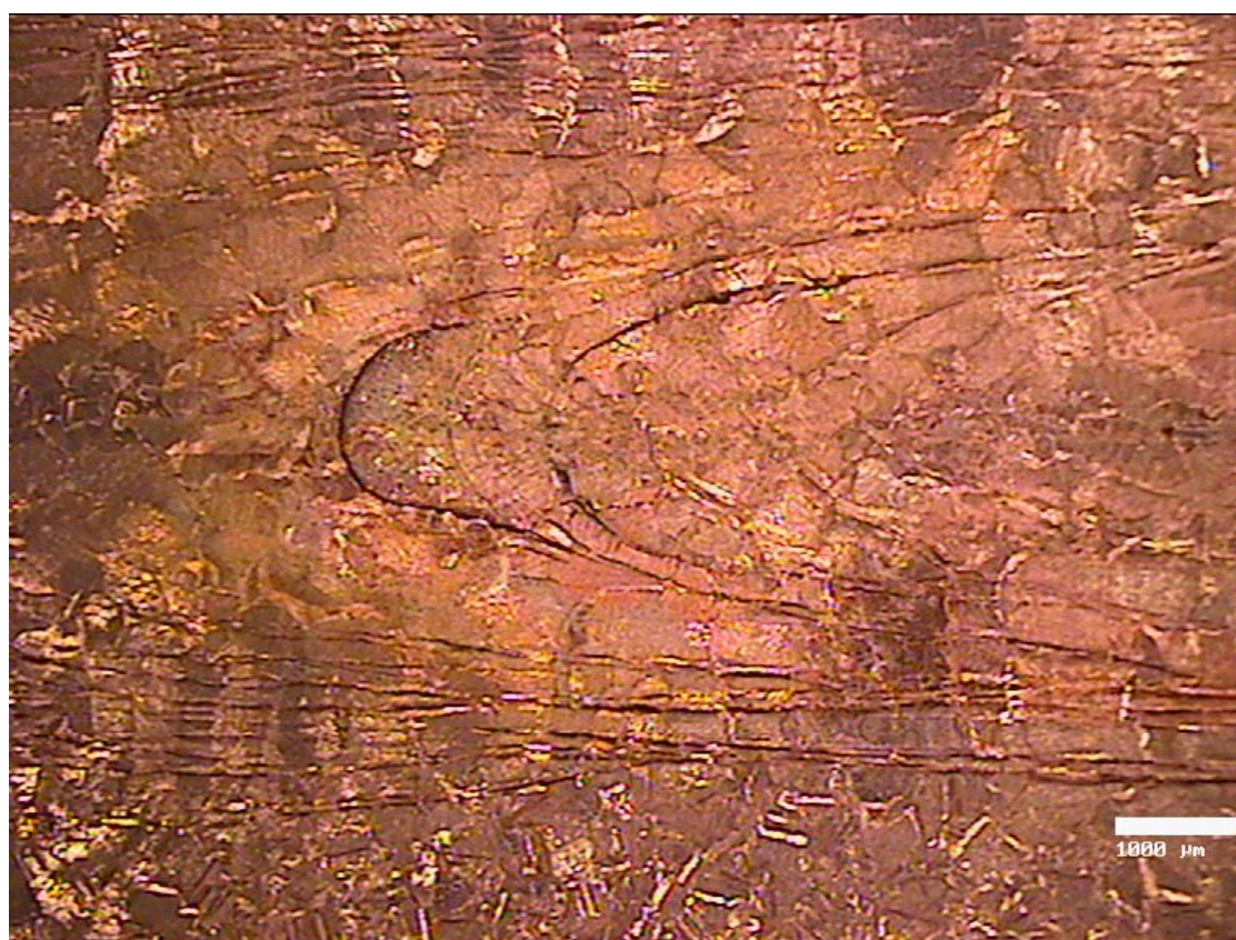
Figure 3-17. Micrograph of sample L017 showing a strong corrosion attack at the root the weld. Small indentions along the grain boundaries can also be observed in this sample.
