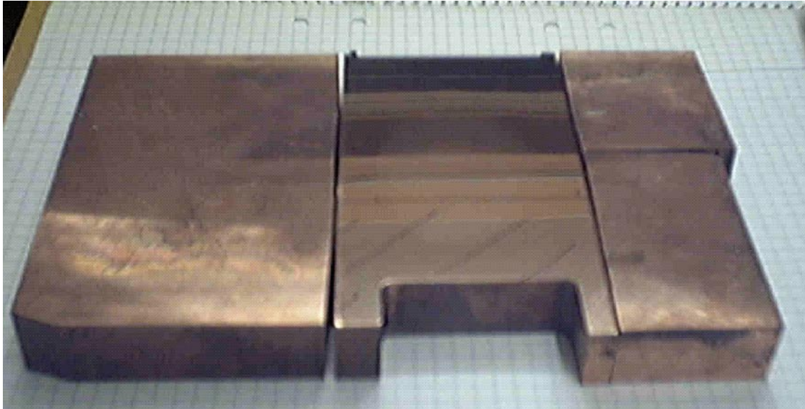
Figure 2-2. Friction stir weld sample. The centerpiece contains the weld in the upper half of the sample.
