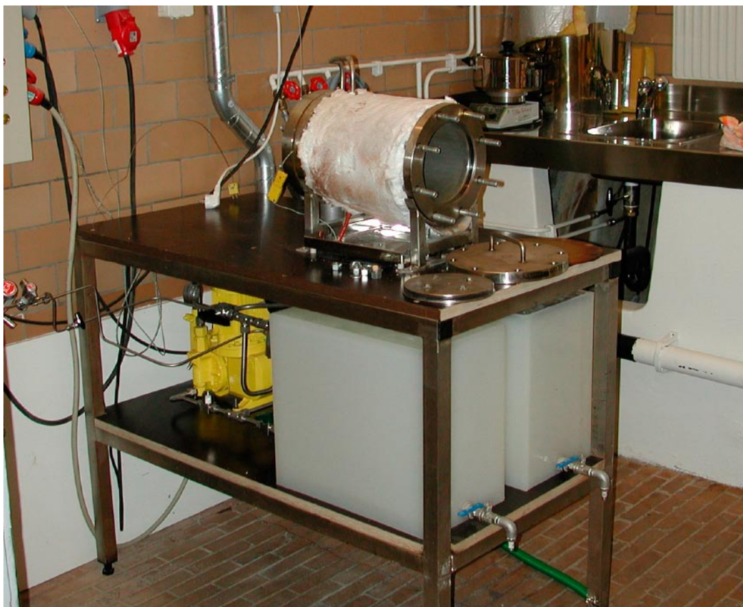
Figure 2-6. Picture of autoclave table with liquid storage tanks and the high pressure pump.
