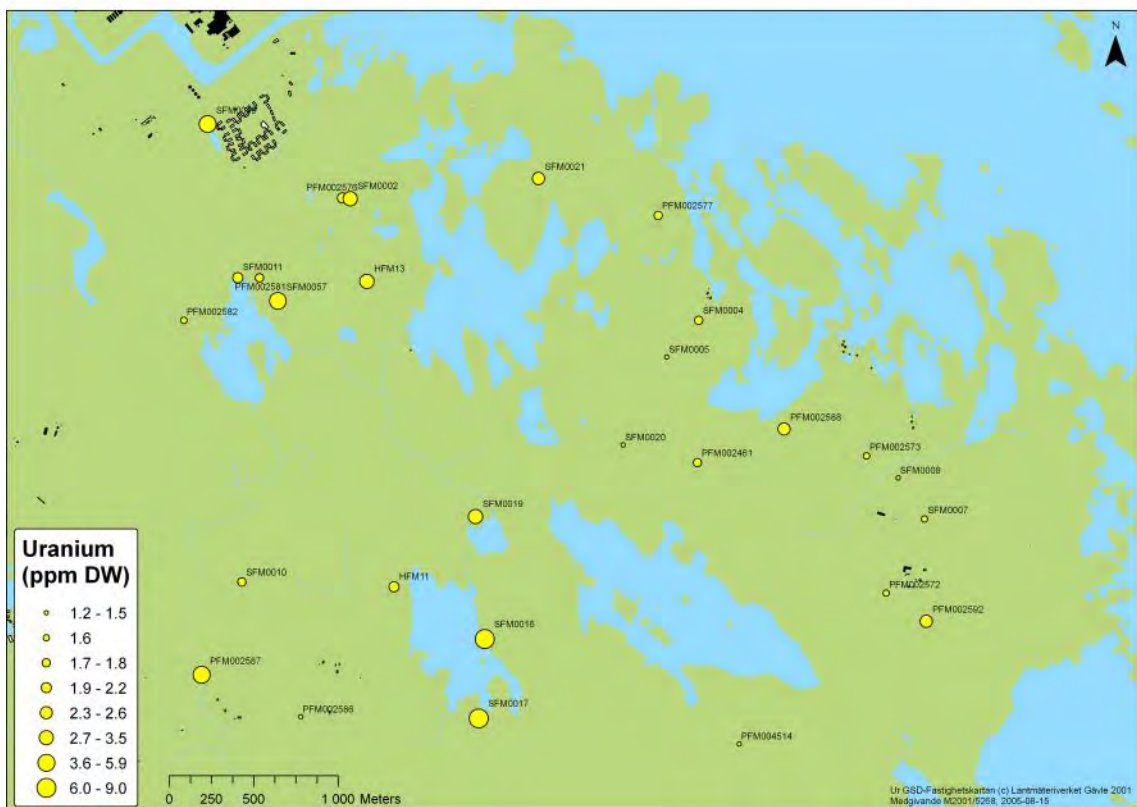
Figure 7-2. Contents of sulphur (upper) and uranium (lower) in till, expressed as ppm of dry weight (DW). It should be noted that the sample plots in the maps represent different stratigraphical positions, thus leading to uncertain comparisons between sites.
