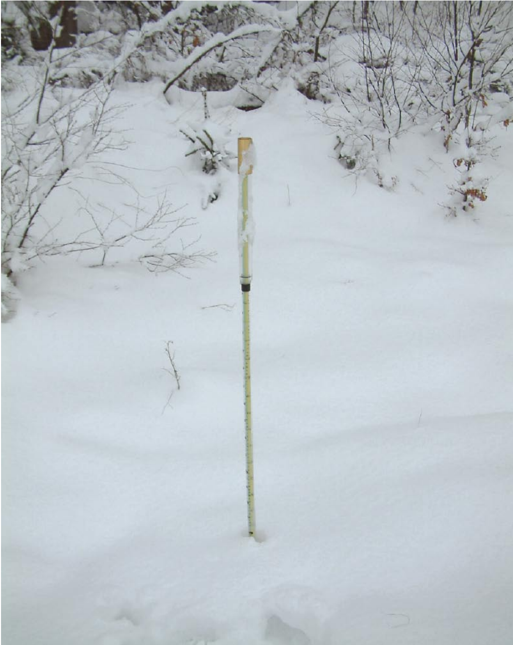
Figure 3-1. Measuring device for registration of depth of frost in the ground at PSM6980.
