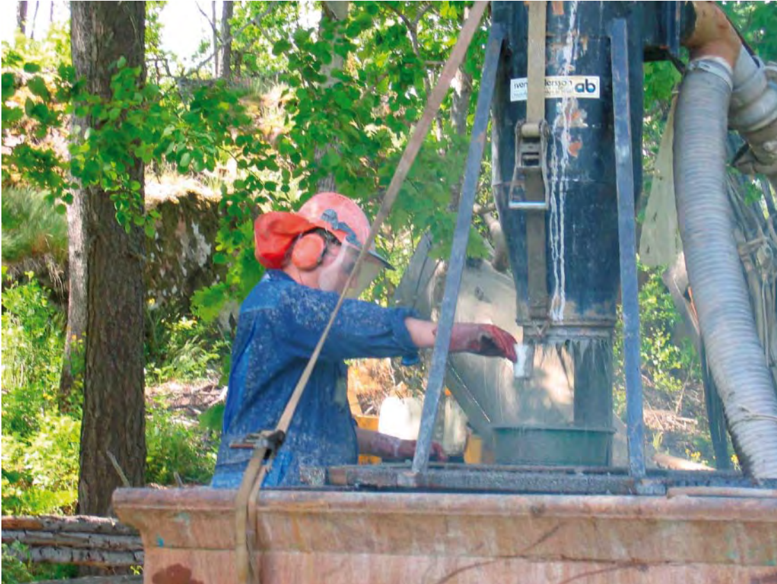
Figure 4-3. Geologist sampling during drilling, drill cuttings are collected in a sieve sitting within the green sieve below the cyclone and return water into small plastic cups, at the drilling site of HLX34 in the north-western part of the Laxemar subarea.
