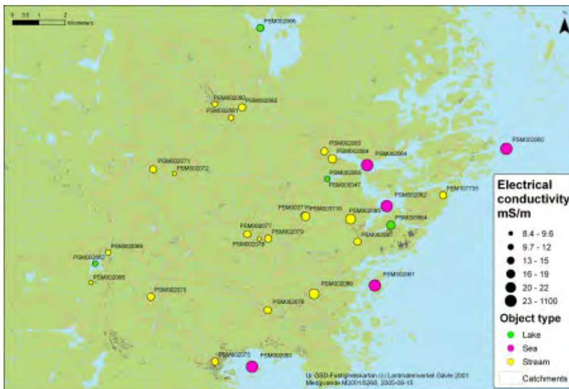
Figure 5-32. Electrical conductivity in surface water in the Simpevarp area (laboratory measurements). Mean value per sampling site.
