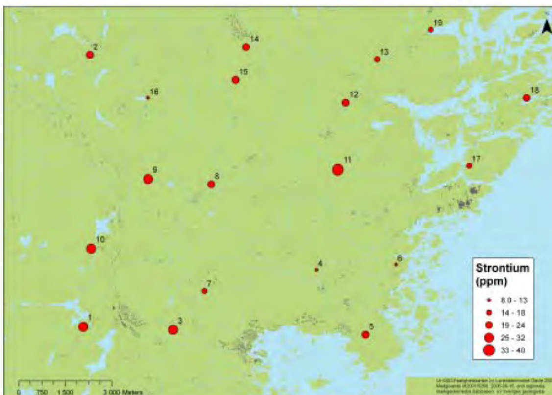
Figure 8-1. Content of calcium (upper) and strontium (lower) in till samples from the Simpevarp area. Extraction by Aqua Regia and ICP-AES analysis. (Ur regionala markgeokemiska databasen. Copyright Sveriges geologiska undersökning (SGU). Medgivande:30-1125/2005.)
