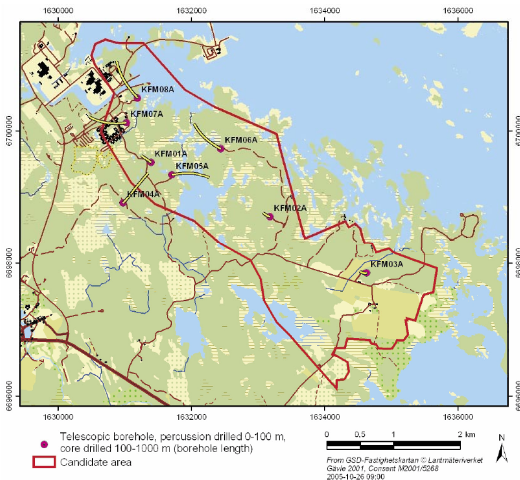
Figure 1-1. Location of all telescopic boreholes drilled up to mid-August 2005 within or close to the Forsmark candidate area. The projection of each borehole on the horizontal plane at top of casing is also shown in the figure.
