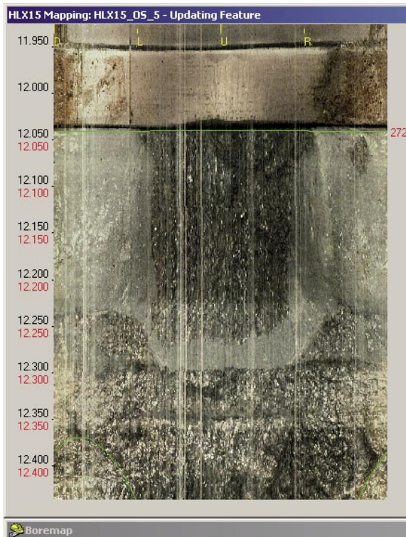
Figure 4-1. BIPS-image as seen in Boremap, borehole HLX15 showing the lowest part of the casing pipe, some rests of concrete from the bottom plug and the borehole wall which is here above ground water level and therefore the visibility of the borehole wall is very limited. Vertical streaks are impurities on protective glass of BIPS-camera and light grey material is lowest part of the concrete seal /1/. Bottom of casing pipe is at 12.04 m.
