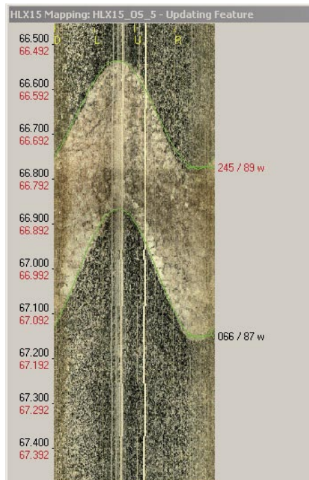
Figure 5-1. BIPS-image as seen in Boremap. Borehole HLX15 showing Quartz monzodiorite cut by white pegmatite. Vertical stripes in the middle of BIPS-image are air-bubbles on the outside of the protective glass of the camera. Horizontal shadow is a result of the automatic blender of the BIPS-camera.
