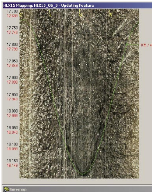
Figure 3-2. BIPS-image as seen in Boremap, borehole HLX15 at 17.6–18.1 m (adjusted length), showing the lack of visibility above the groundwater level, wet and glittering borehole walls. Vertical lines are impurities from protective glass on BIPS-camera and lighter colour on the sides is mud on the lower side of borehole wall. One probable open fracture is marked (green line).
