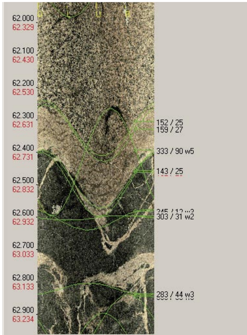
Figure 5-4. BIPS-image as seen in Boremap, borehole HLX28 showing weakly oxidised quartz monzodiorite cut by fine-grained granite dyke and containing veined and fine-grained diorite-gabbro enclave (fragment).
