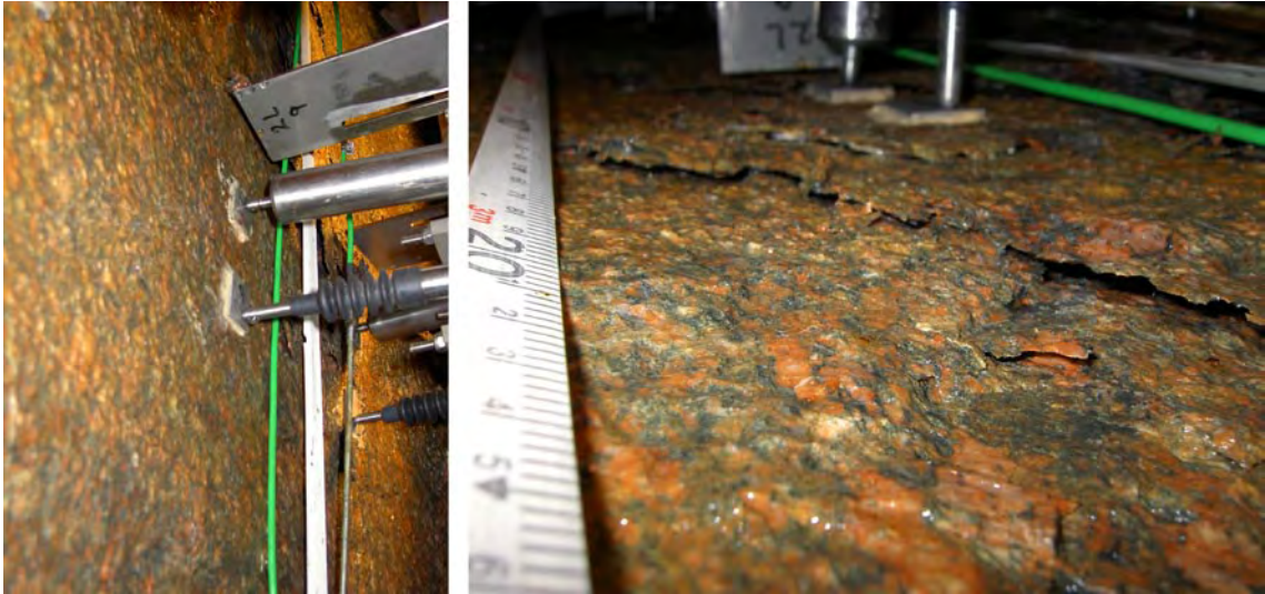
Figure 6-3. Photograph of instrument position #9 was taken on June 2 nd (left) and on June 16 th (right).
