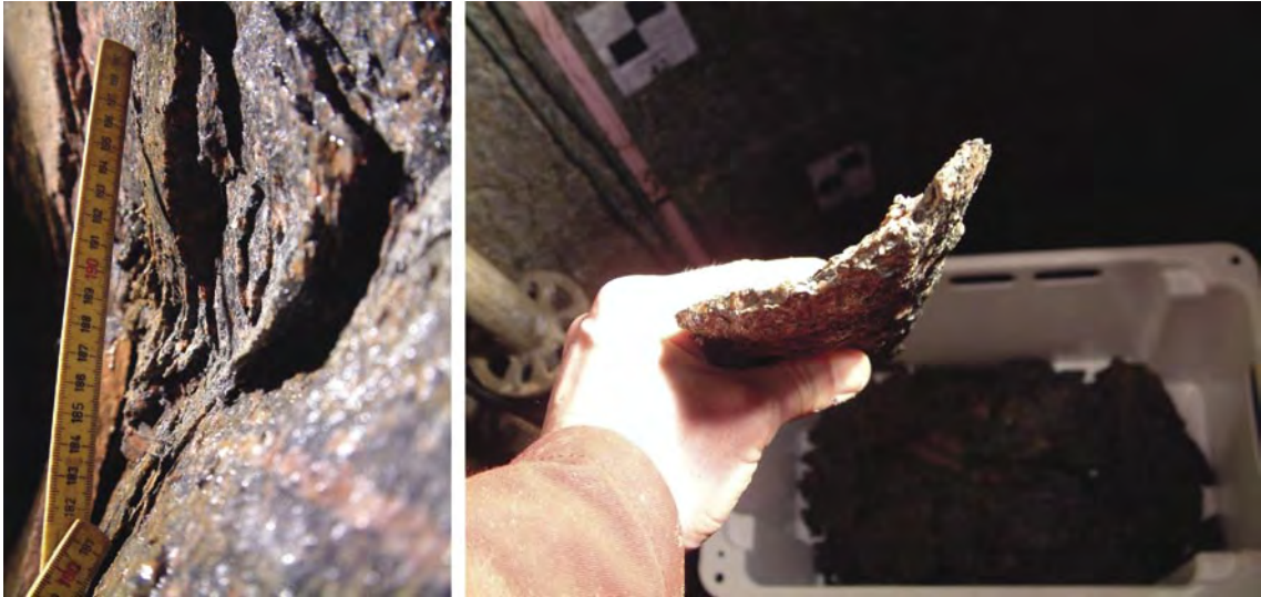
Figure 5-68. Photograph of the location of the arched chip and the chip itself.
