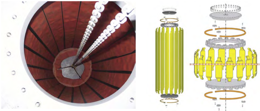
Figure 3-6. Left: the confinement equipment that held the rubber bladder membrane; right: Microstation drawing of the equipment. The load-bearing textile straps are orange/red in the construction and yellow in the drawing.
