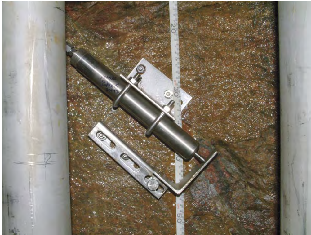
Figure 3-16. Short range LVDT placed over the shear zone.
