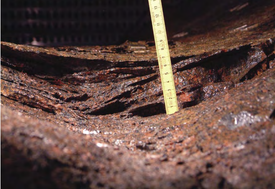
Figure 5-62. Photograph of the smooth arched notch at a depth of 3.7 m.
