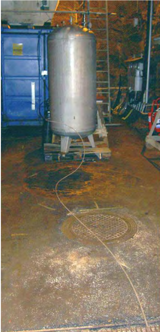
Figure 3-9. Photograph of the pressure vessel connected to a gas cylinder. The flexible Tecalan tube in the photograph is connected to the bladder via the top steel lid and ensures the pressure in the bladder.
