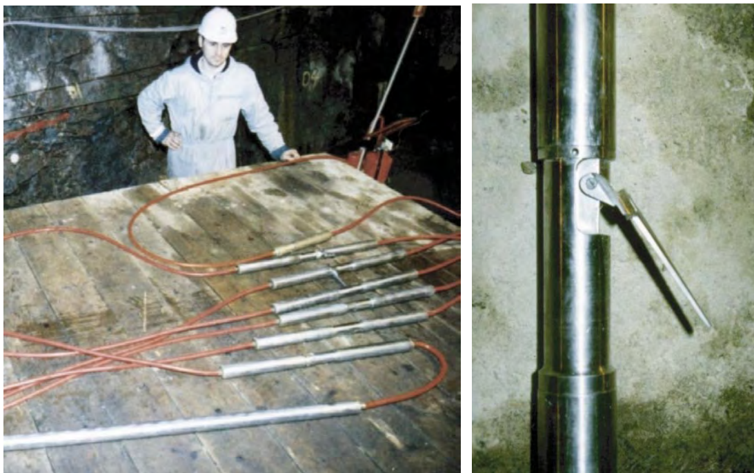
Figure 7-9. The R8-XYZ geophones, equipped with side-arms for clamping, used for the VSP surveys from turn 2. DC motors activate the arms and the clamping control is independent for each unit.
