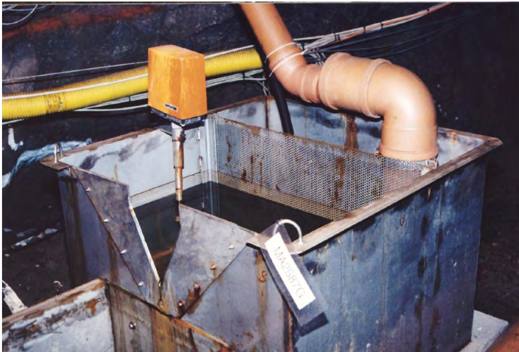
Figure 11-8. Installation for electrical conductivity measurements in a Thomson weir, representing the conductivity of water flowing in from a tunnel interval.
