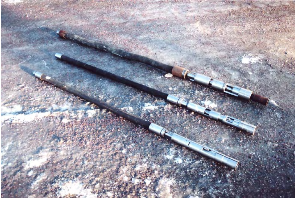
Figure 5-7. Packer equipment used for grout injection during core drilling. The uppermost for 76 mm boreholes (single packer injection) and the lower for 56 mm boreholes (single packer and double packer injection).
