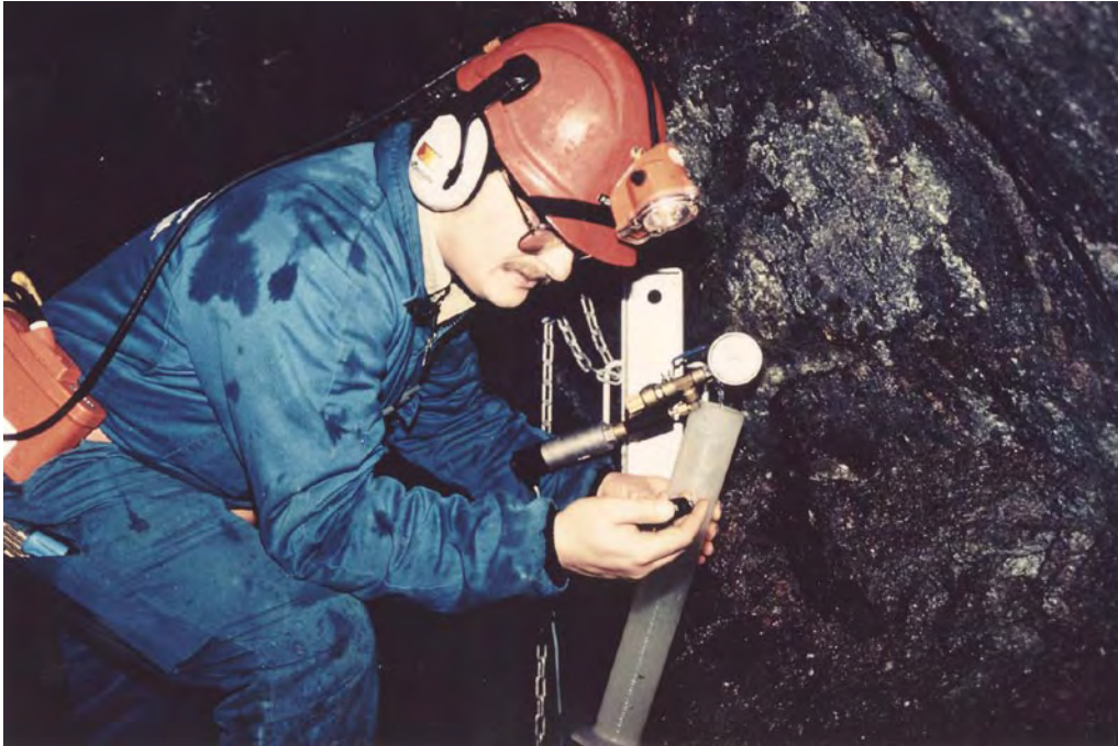
Figure 8-2. Pressure build-up tests just behind the tunnel front during drill and blast tunnelling.
