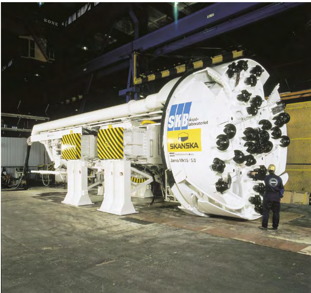
Figure 2-3. The TBM machine in the assembly hall before TBM tunnelling start.
