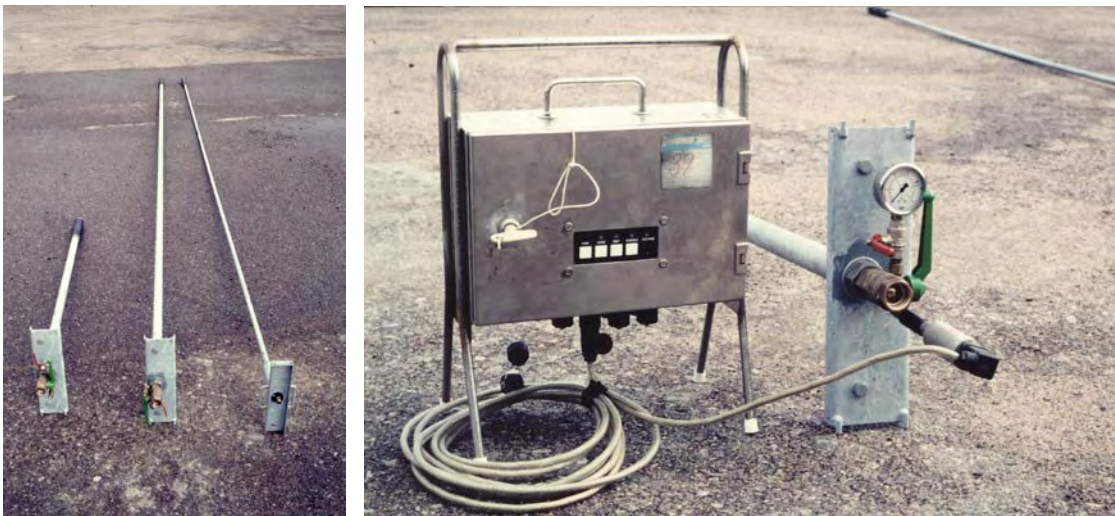
Figure 8-3. Equipment for pressure build-up tests in probe holes. Left: Packers for pressure build-up tests in probe holes. The long “standard” packer to the right, long packer for high flow in the middle and a short packer for severe installations in curved holes. Right: Borre MDL data logger and pressure transducer mounted to the BAT rubber disc connection of the valve arrangement.
