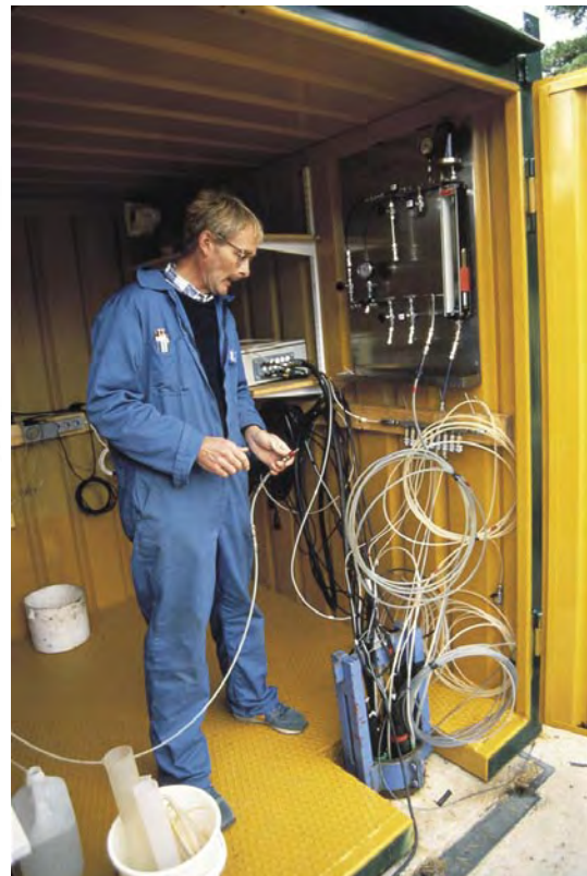
Figure 8-16. Principal outline of borehole equipment for dilution measurements.
