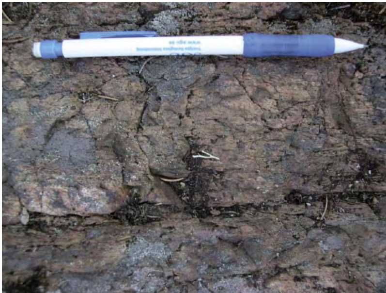
Figure 5-22. Strongly deformed, mylonitic Ävrö granite within the northern branch of the so-called Äspö shear zone (PSM003826).
