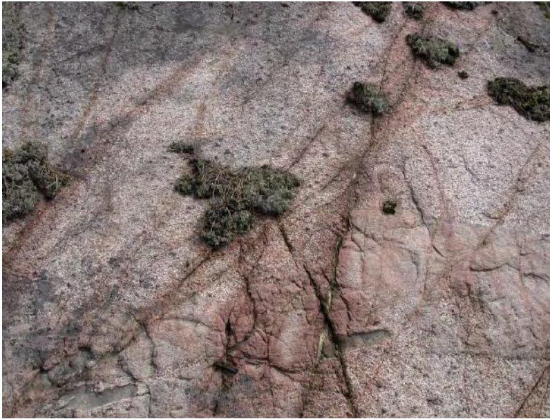
Figure 5-27. Red staining (oxidation) around and along fractures in Ävrö granite and fine- to medium-grained gnaite (PSM004403).
