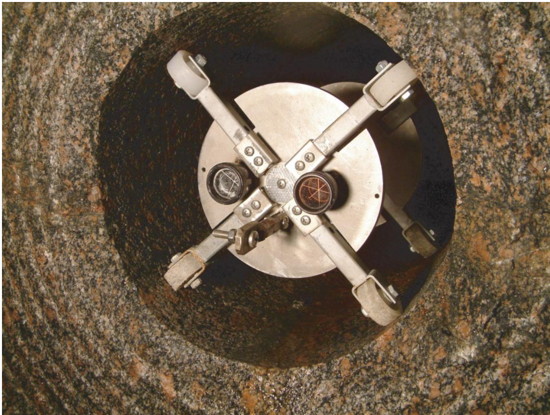
Figure 5-16. Device used for measuring the straightness of the pilot hole.
