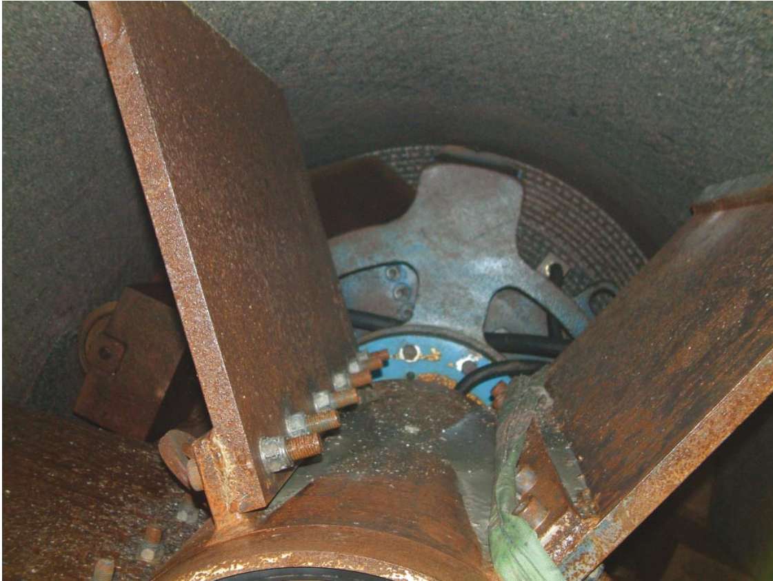
Figure 5-13. Reamer head stabilizer.
