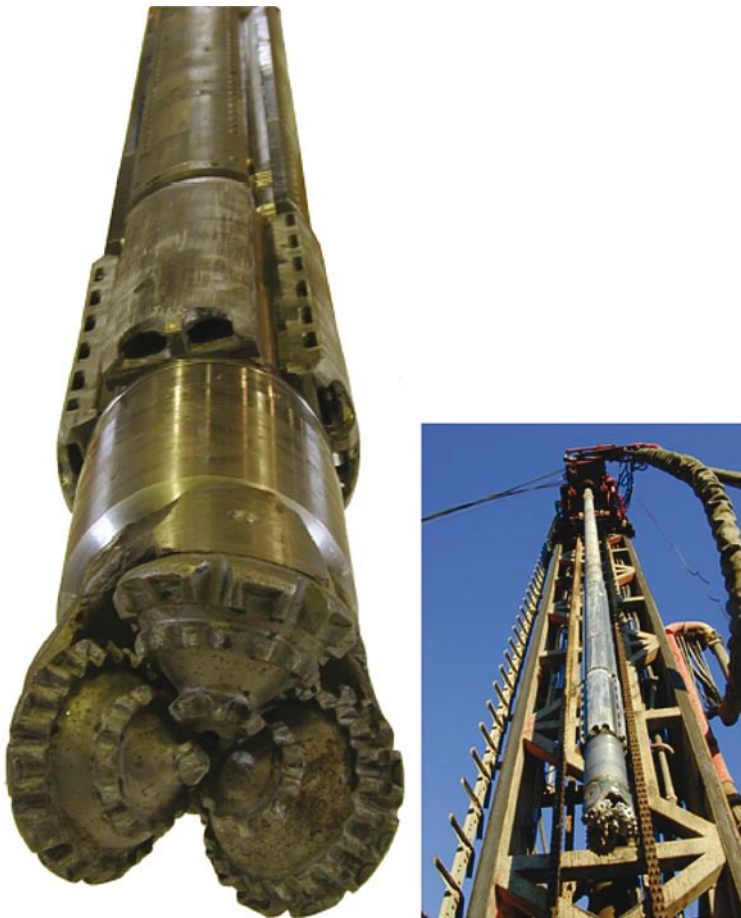
Figure 5-5. Detail showing the drill bit and the Rotary Drilling System.
