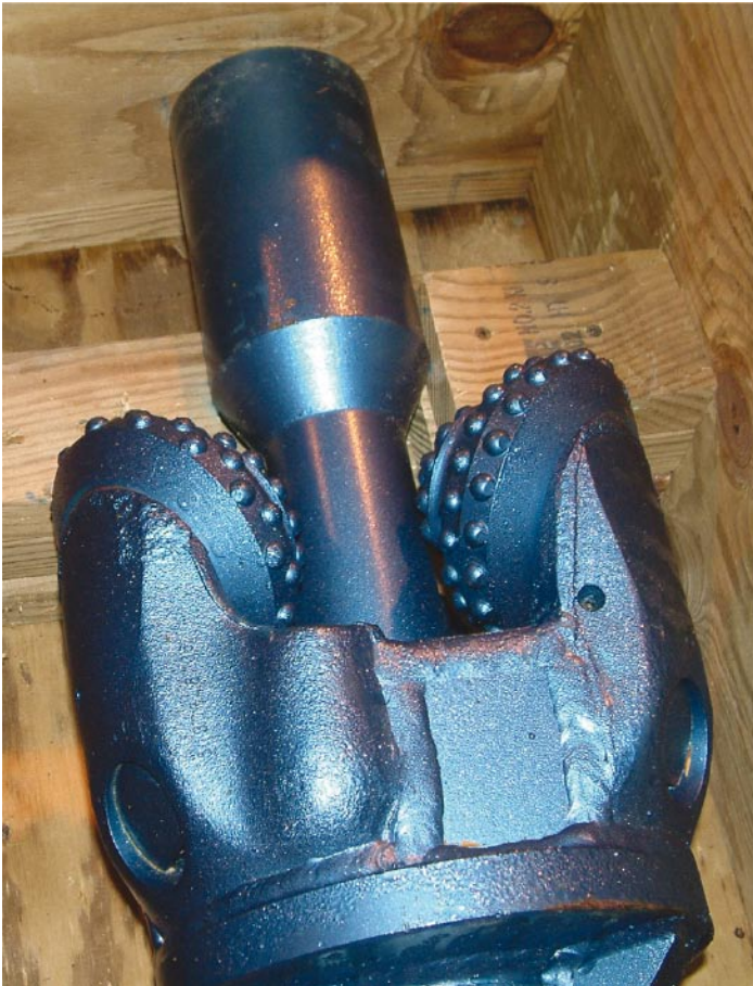
Figure 5-9. Drill bit planned to be used when the pilot hole is reamed from 152 mm to 279 mm.
