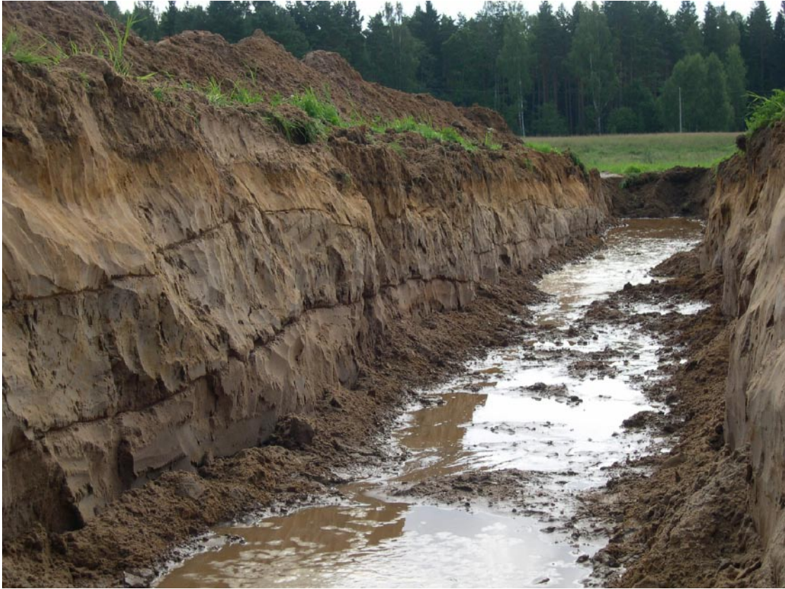
Figure 5-13. Trench dug at Malmgrava (E2 in Figure 1-1) along the Fårbo esker some 30 km northwest of Simpevarp. Although raised above the sea very shortly after deposition and, thus, entirely water-logged during only a few years or decades, the sandy-silty deposits have to some degree, due to a fairly high groundwater table, remained susceptible to seismically induced deformation.
