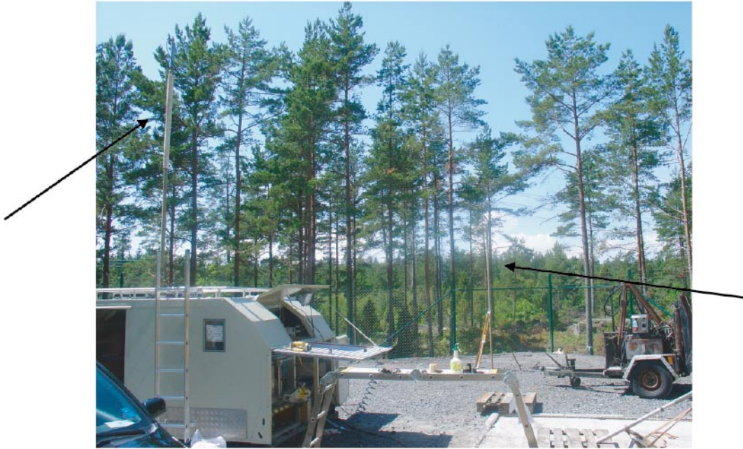
Figure 4-2. Test of the functionality of the directional antenna at drill site KLX07, Laxemar. The receiver antenna is mounted on the roof of the container and the transmitters held by a tripod.
