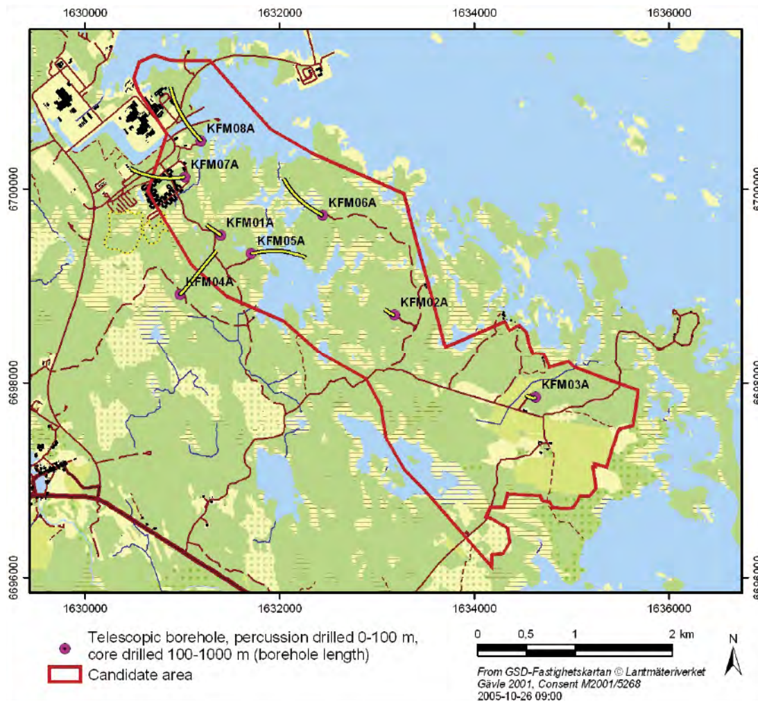
Figure 1-1. Location of all telescopic boreholes drilled up to now (October 2005) within or close to the Forsmark candidate area. The projection of each borehole on the horizontal plane at top of casing is also shown in the figure.
