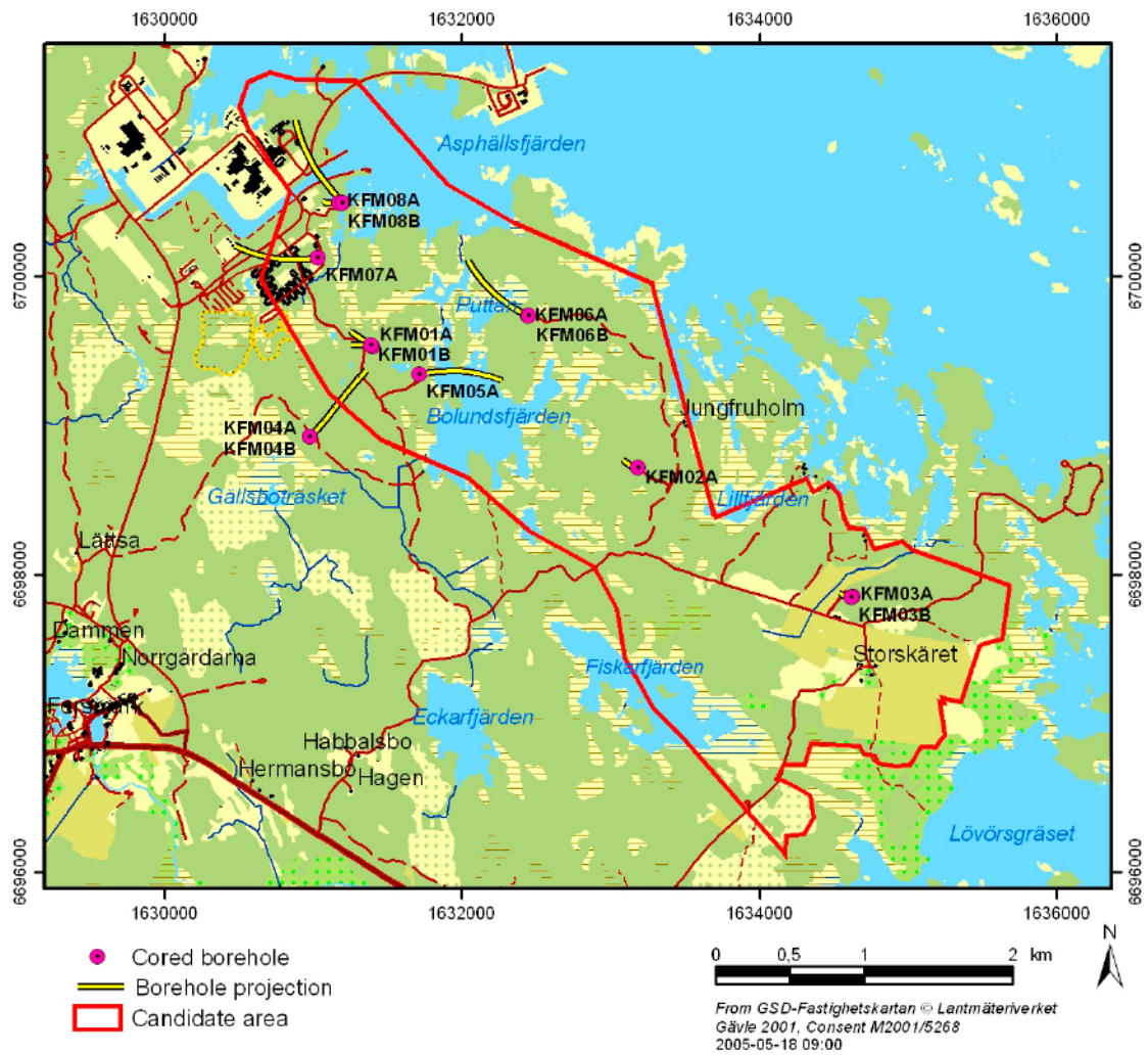
Figure 1-1. The investigation area at Forsmark (approximately the area inside the black square) including the candidate area selected for more detailed investigations. The collarings of the deep telescopic boreholes, KFM01A to KFM08B, are marked with red circles. The projection of the boreholes on the horizontal plane at top of casing is also shown in the figure.
