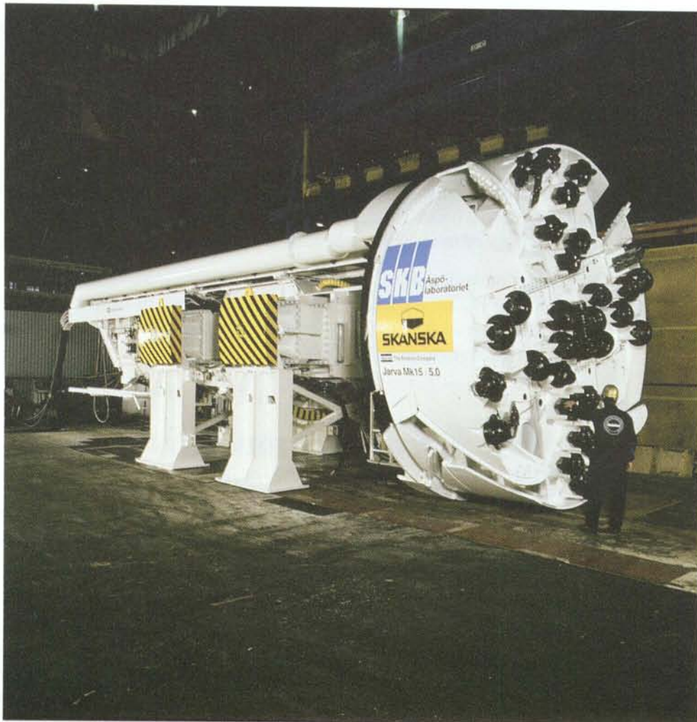
Figure 8-1. The TBM is a 5 m diameter ATLAS COPCO JARVA MK15.
