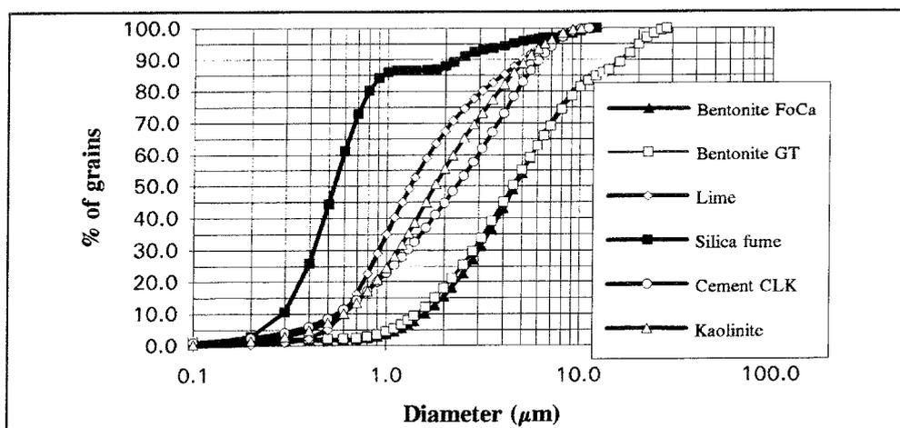
Figure 4.5-3. Grainsize-distribution curves of sealants.
