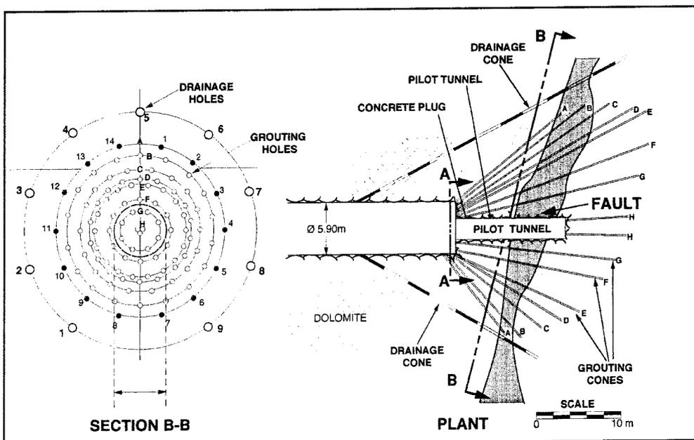
Figure 2.4-7. Final phase. Removal of plug and boring through fault.
