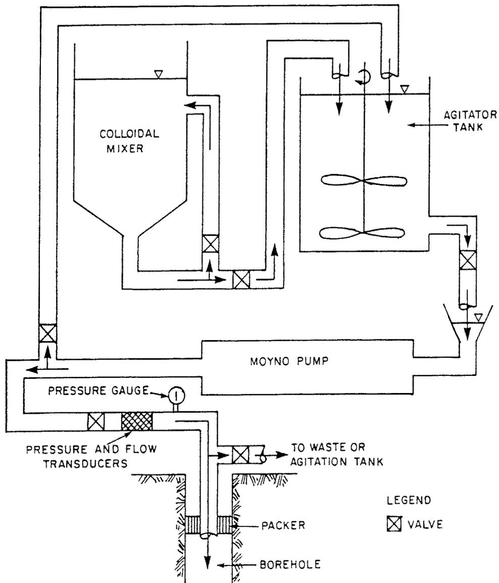
**Figure 4.3-4. Schematic arrangement of grouting plant.**
