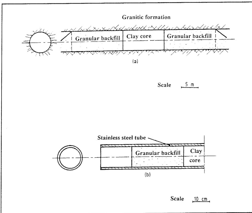
**Figure 4.6-1.** Clay core dam schematic layout and its scale model
