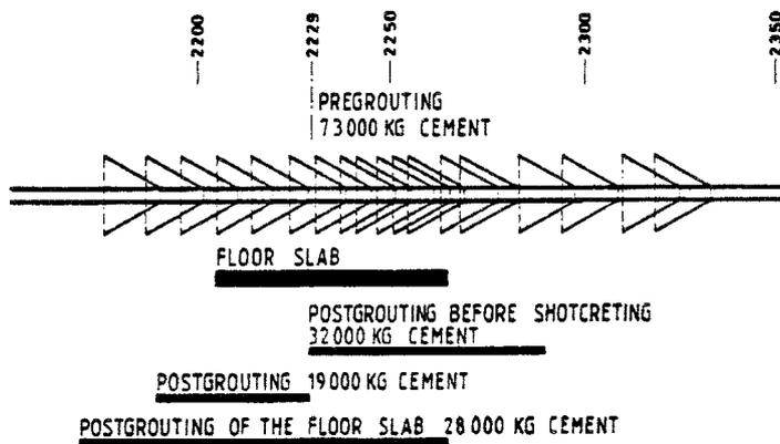
*Figure 2.2-3. Sea Sewer. Grouted area and number of pregrouting rings.*
