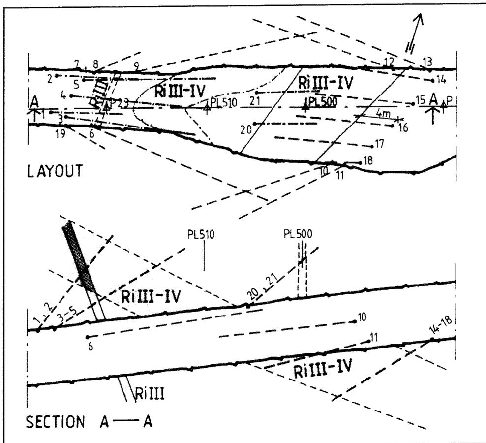
Figure 2.2-4. VLJ Repository. Grouting plan of the RC zone in the access tunnel.
