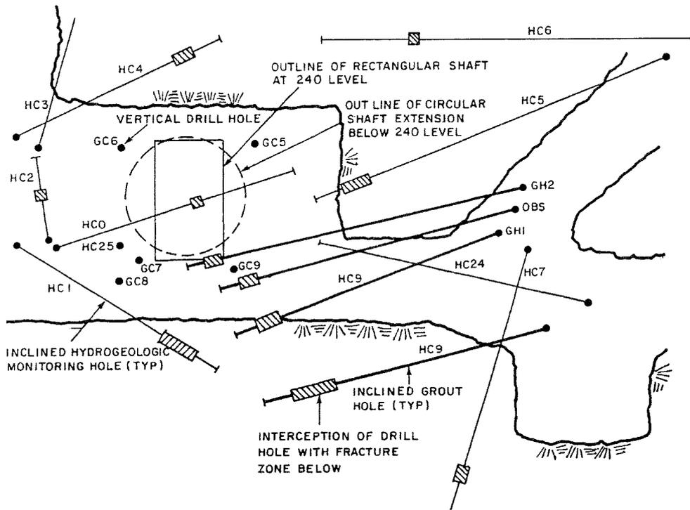
Figure 4.3-3. Plan of drill holes for URL grout trials.
