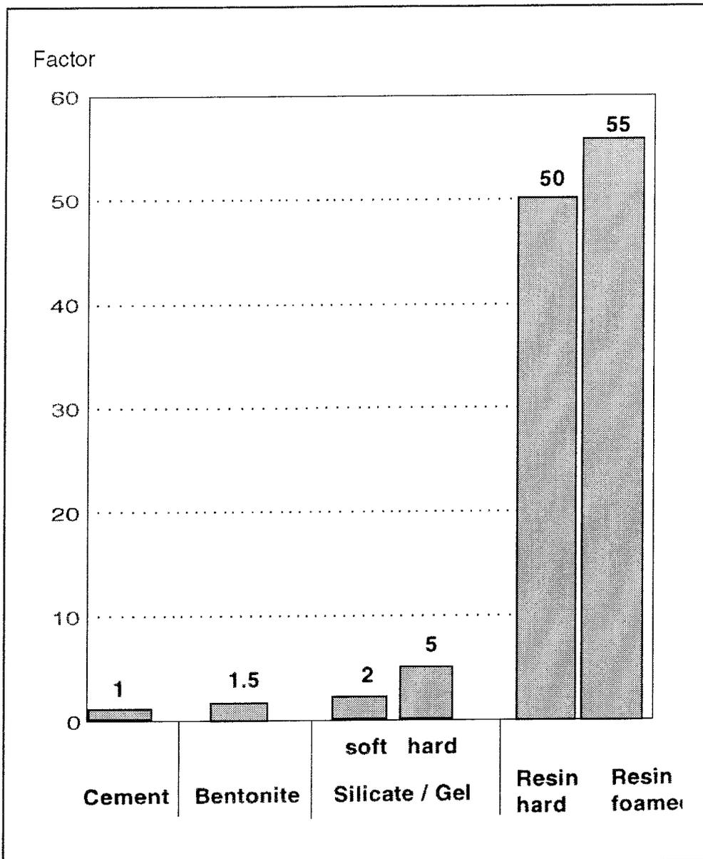
Figure 2.4-2. Basic costs per kg of grouting material.
