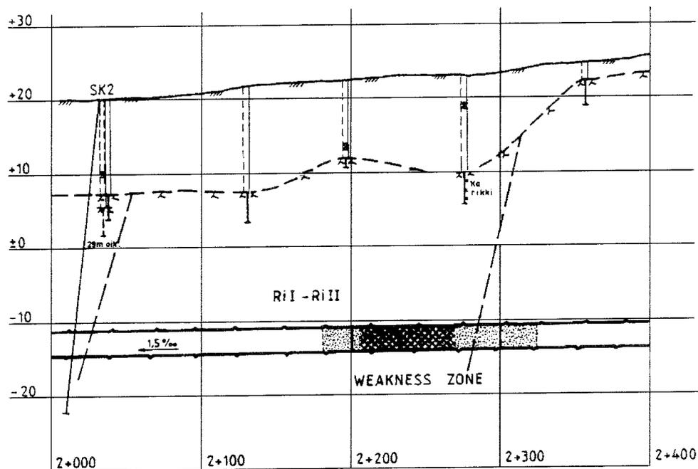
*Figure 2.2-1. Longitudinal section of the Sea Sewer sewage tunnel in the area of the Harjusuo zone of weakness.*
