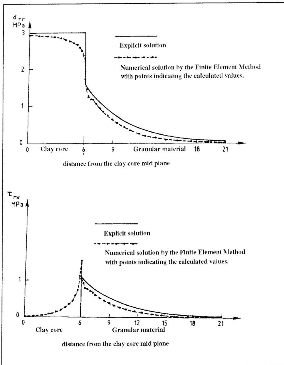
**Figure 4.6-2.** Normal and tangential stress components at the gallery wall as a function of the distance from the clay core dam mid plane.
