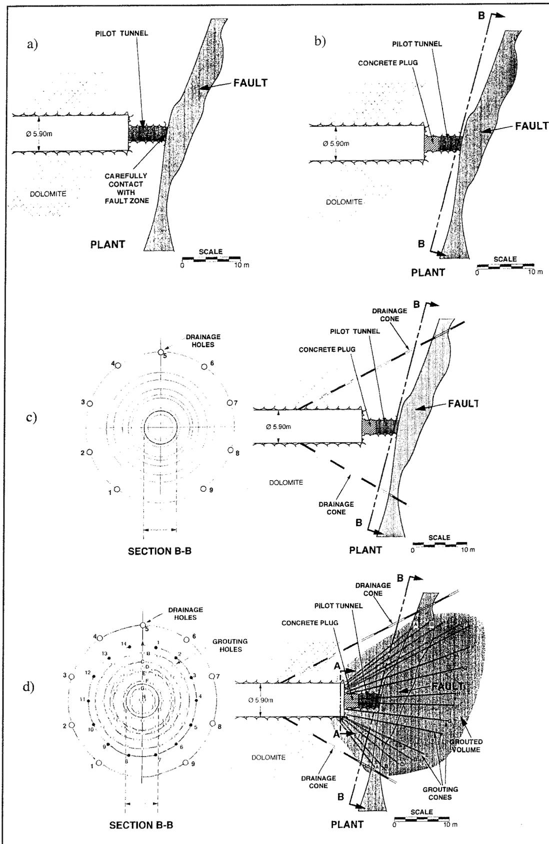
Figure 2.4-6a. Final phase. First contact with fault zone.
