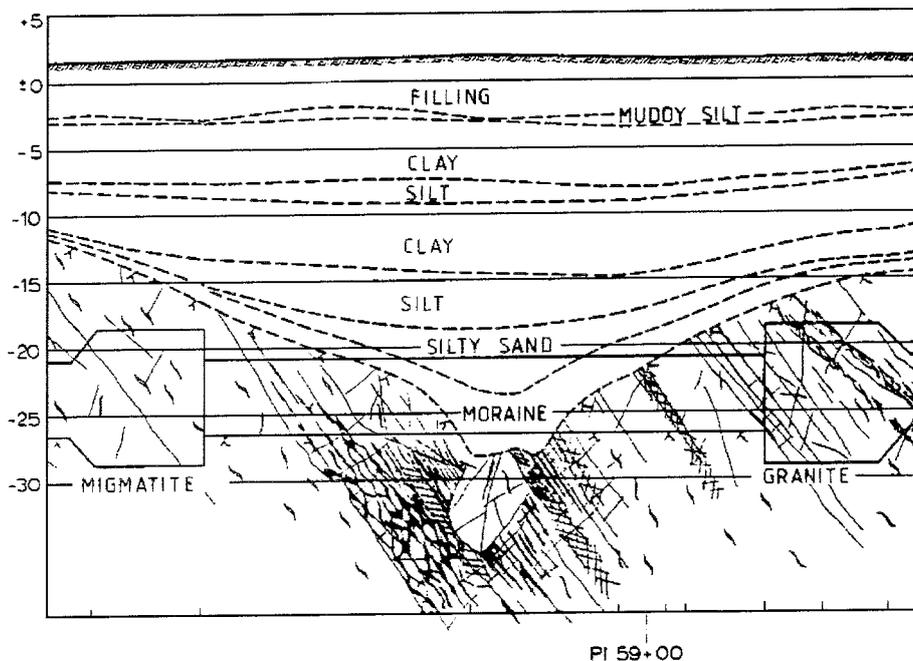
Figure 2.2-6. Soil and rock conditions of the Kluuvi Cleft /Hartikainen et al., 1978/.
