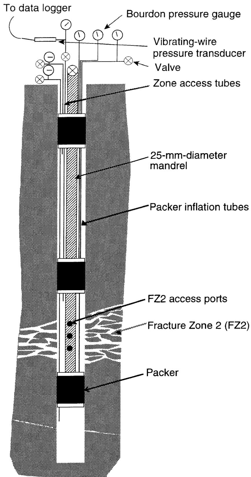
**Figure 2.1-4.** Multiple-packer monitoring system used to characterise Fracture Zone 2.
