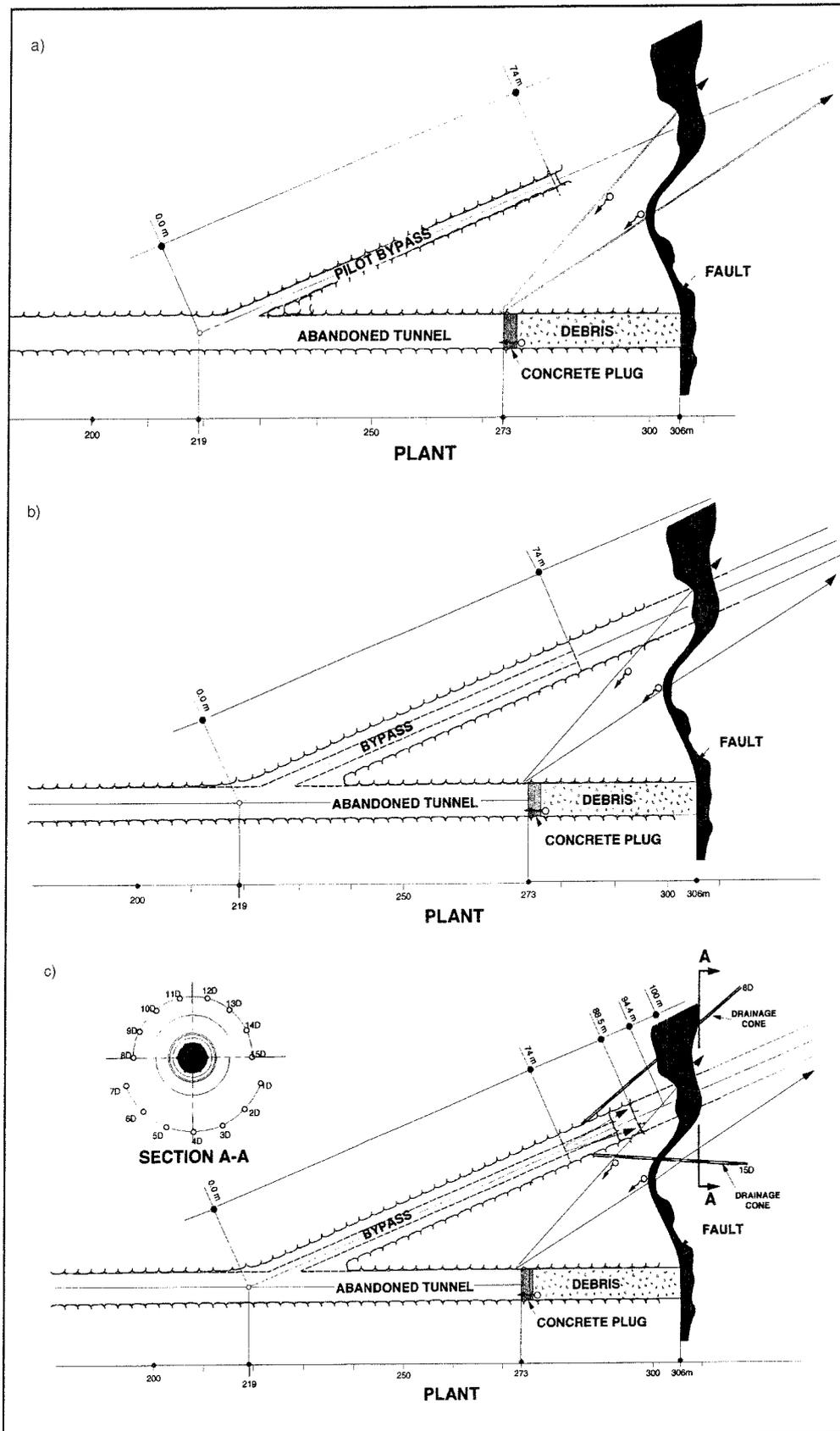
Figure 2.4-4a. Start of the pilot bypass tunnel.
