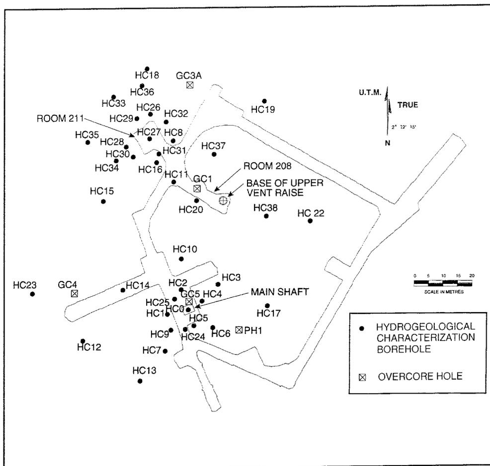
**Figure 2.1-3.** Locations of intersections of hydrogeological characterization and overcore stress determination boreholes with Fracture Zone 2, superimposed on a plan view of the 240 m level.
