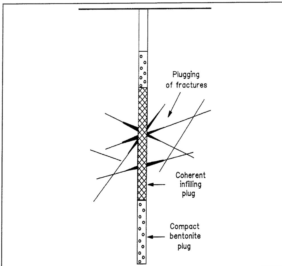
Figure 4.5-2. Tailor-made borehole sealing.
