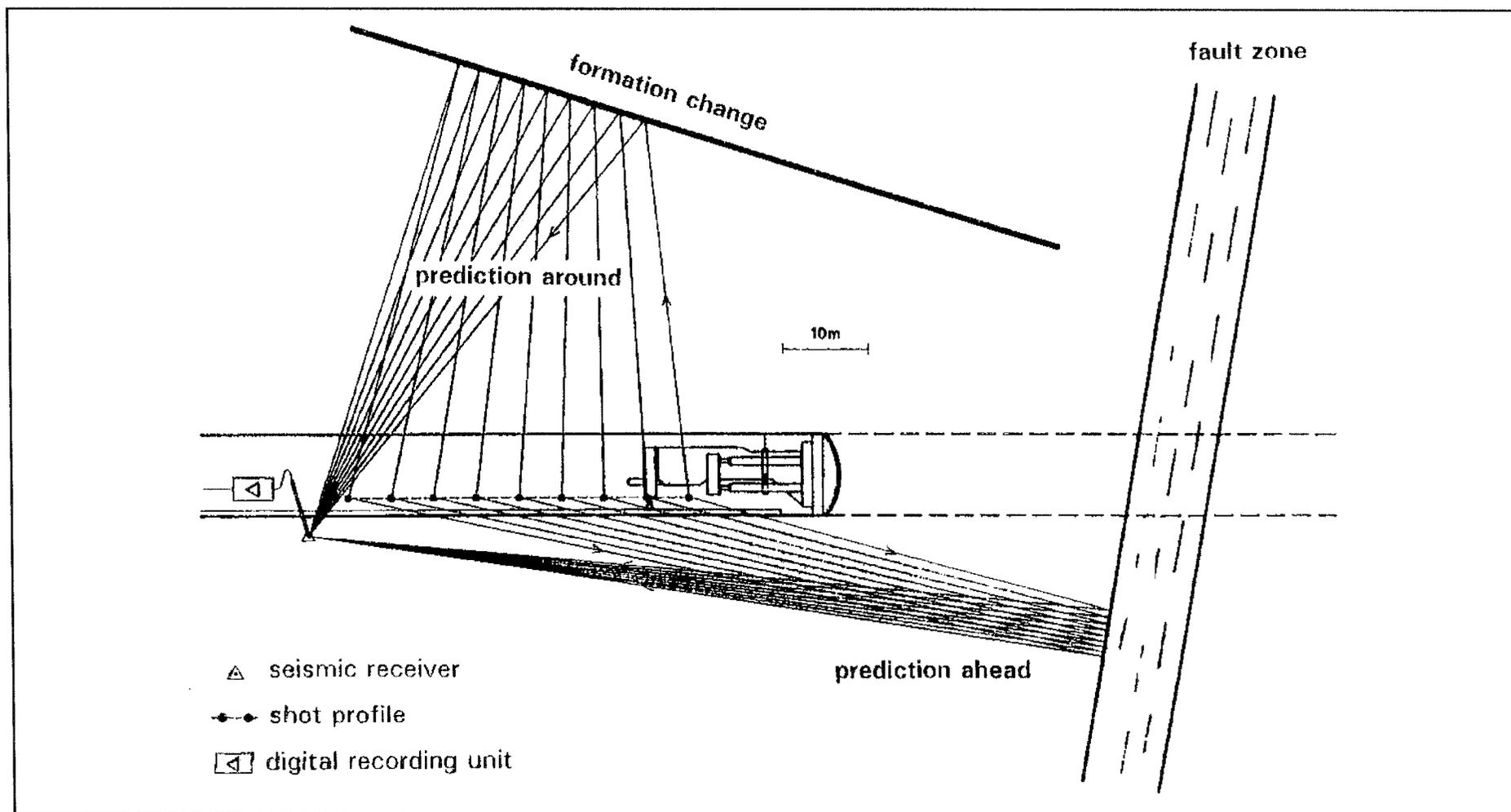
Figure 2.4-1. Measurement principle of seismic prediction ahead of the tunnel face.
