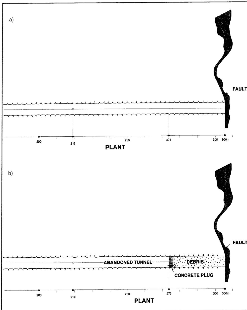
*Figure 2.4-3a. Normal tunnel excavation without knowledge of the incoming fault.*
