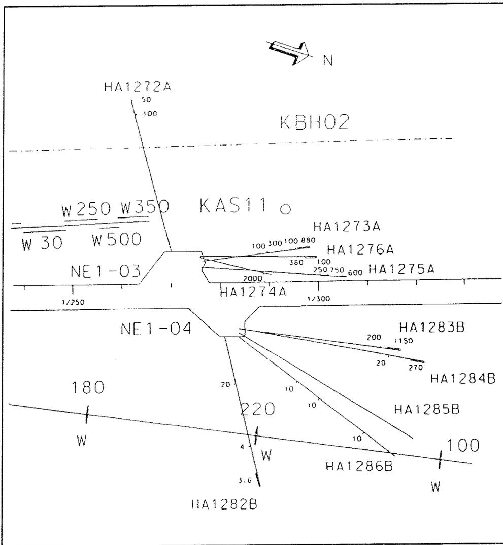
**Figure 2.3-2.** Positions of the percussion boreholes in niches NE1-03 and NE1-04. The figures on the boreholes are the inflow of water in l/min.
