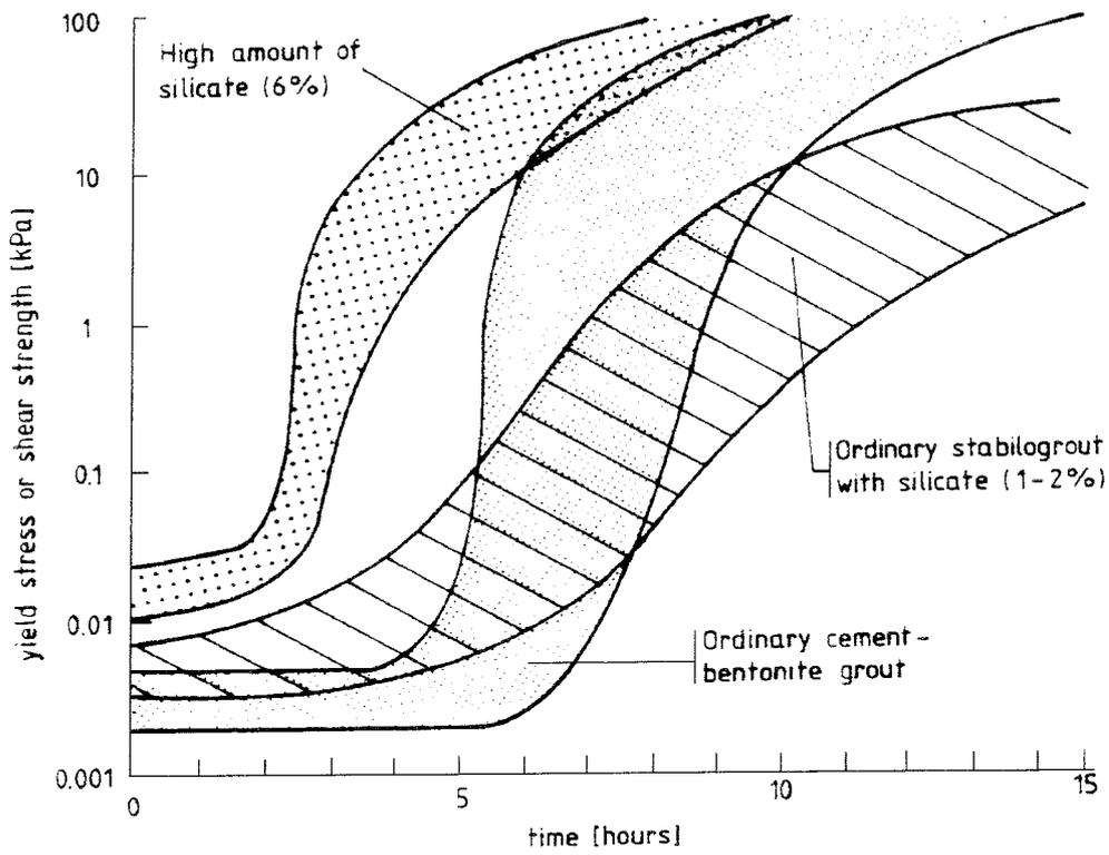
Figure 2.3-3. The effect of silicate.
