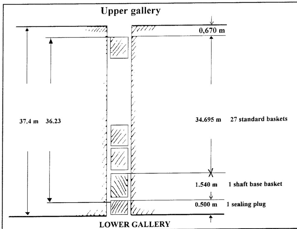
Figure 4.4-3. Specification of the stacking.
