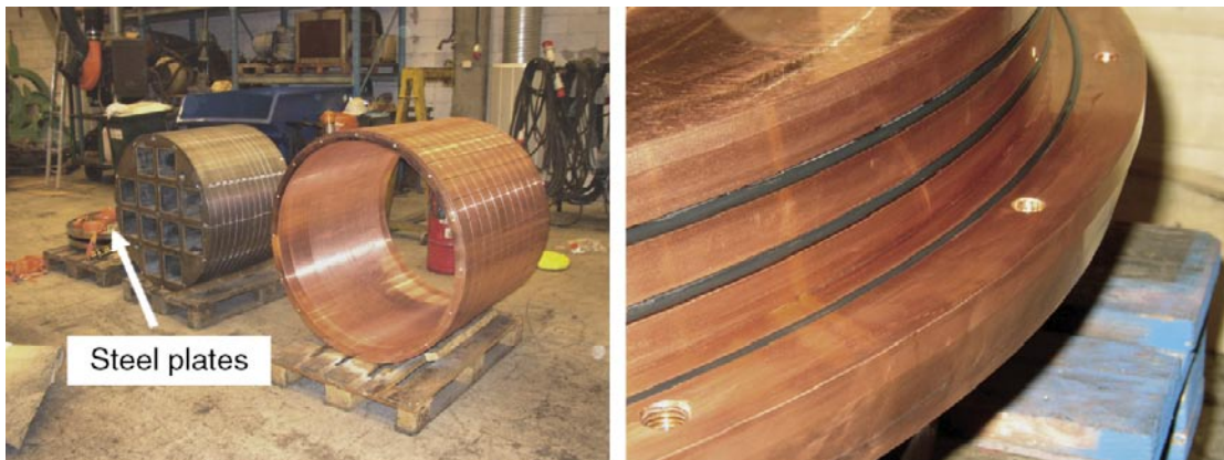
Figure 2-2. a) Cast iron insert and copper tube cut to specified dimensions and machined before assembly b) detail of copper lid with O-rings.
