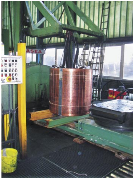
Figure 3-2. a) Mock-up ready for testing b) mock-up inserted into the cold isostatic press.
