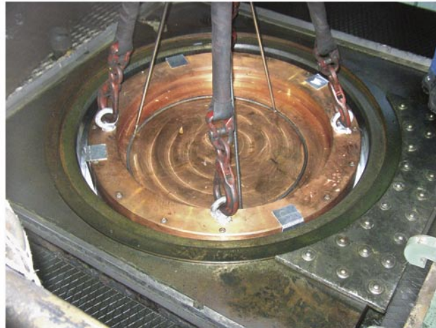
Figure 3-2. a) Mock-up ready for testing b) mock-up inserted into the cold isostatic press.
