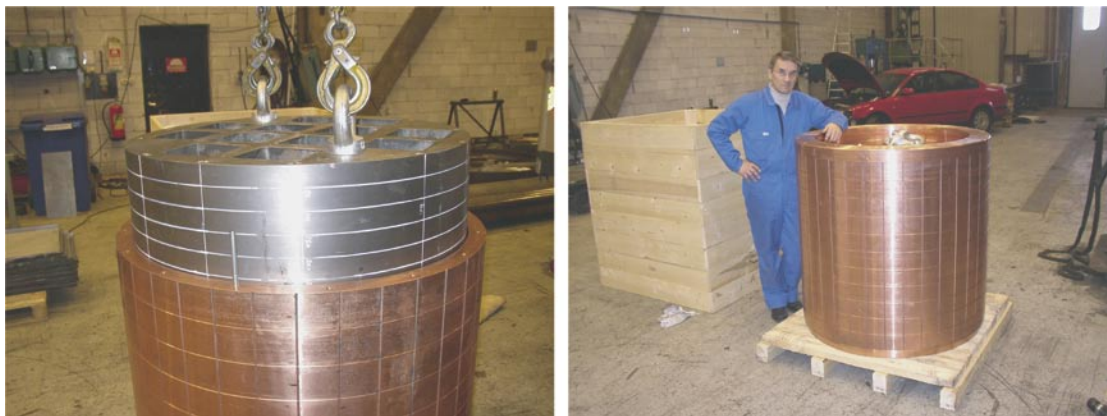
Figure 2-3. a) Cast iron insert being inserted into the copper tube and b) assembled mock-up.
