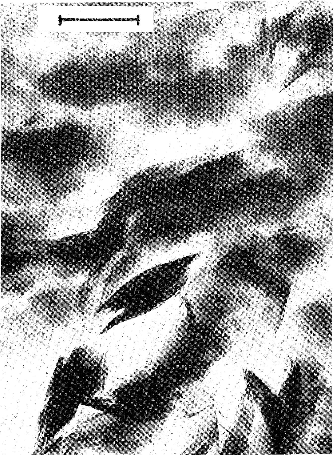
Figure 2-34 TEM photo showing dense I/S aggregates and presumed neoformed illite in large pores (uppermost part). Scale is 0.1 \mu\text{m} (51)
