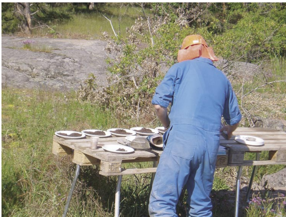
Figure 4-3. Sampling and preliminary logging by the drill site geologist of samples of rock chip drill cuttings at the drill site for borehole HAV11 on the south-eastern coastline of the island Åvrö.
