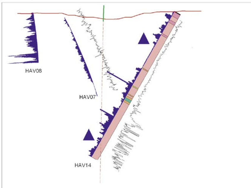
Figure 6-4. Profile of boreholes HAV11 and HAV14. Shown with preliminary geological results (soil is shown in black), magnetic susceptibility (blue bars) and drilling penetration time (black line). Positions for water inflow are indicated by blue triangles. Red line shows ground/water surface. Green line shows position of investigated lineament based on results from surface investigations, with dashed line indicating possible intersection with borehole. Profiles of boreholes HAV07 and HAV08 are shown with HAV14, but HAV08 only shows susceptibility, while HAV07 shows both susceptibility and penetration time, but neither has any known geological data. For mutual positions see plan map in Figure 6-3.
