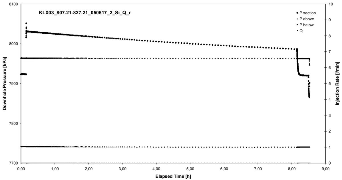
Pressure and flow rate vs. time; cartesian plot, long term measured over night
