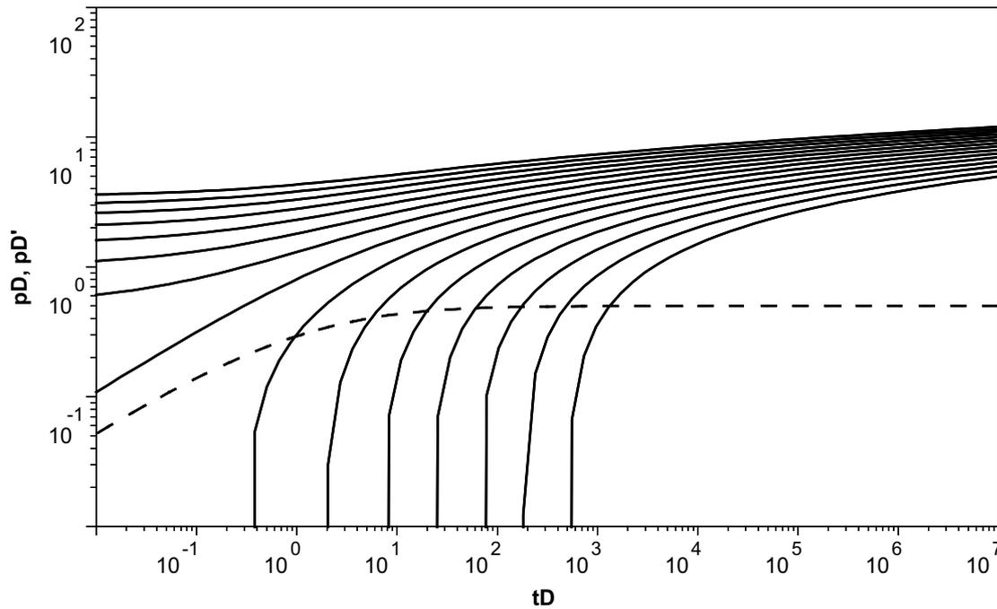
*Figure 5-3. Deconvolution type curve set for pulse and slug test analysis.*
