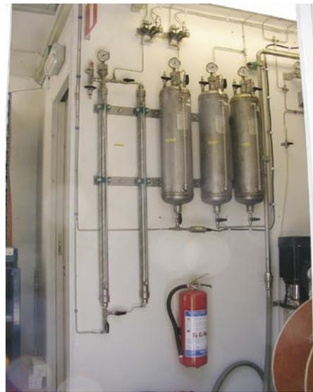
**Photo 4.** Pressure vessels for test valve, packers and injection.
