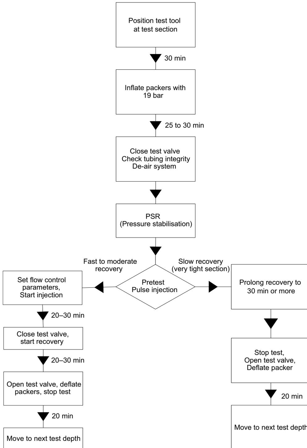
**Figure 5-1.** Flow chart for test performance.
