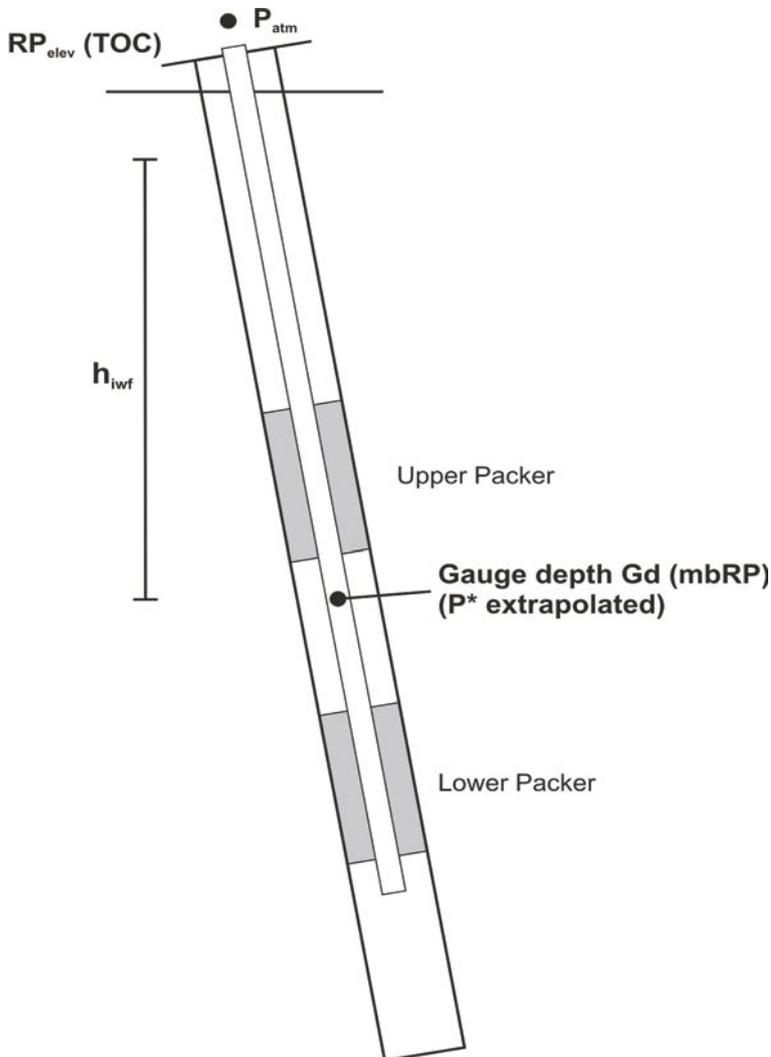
*Figure 5-4. Schematic methodologies for calculation of the freshwater head.*
