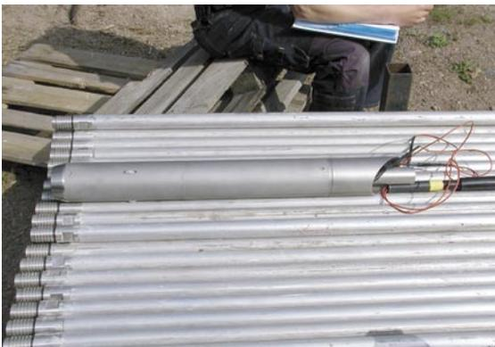
**Photo 5.** Positioner, bottom end of down-hole string.
