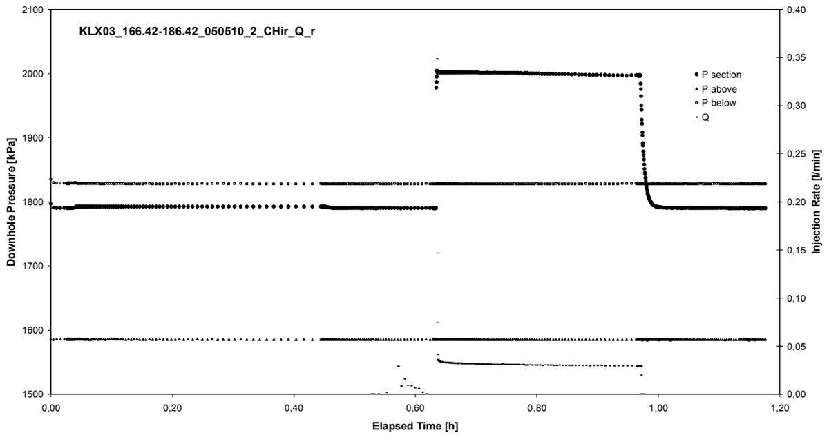
Pressure and flow rate vs. time; cartesian plot (analysed)
