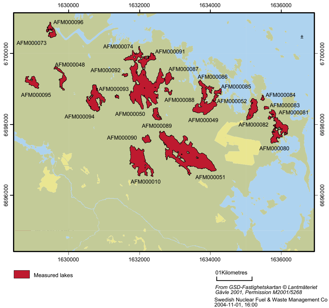
Figure 3-15. Lakes where the SKB DEM points are replaced by measured values. For all other lakes the elevation was set to the mean value from the SKB DEM.
