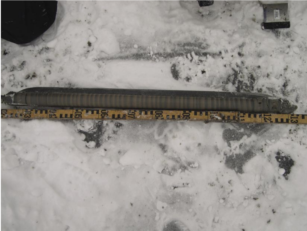
Figure 3-26. Example of a sediment sample collected from the bottom of Lake Eckarfjärden. The corer collects 1 m long sediment sequence that is inspected and described in the field. The corer is hand driven and is used in soft deposits such as gyttja, clay and peat. The investigated sediments do not include coarse-grained deposits such as till.
