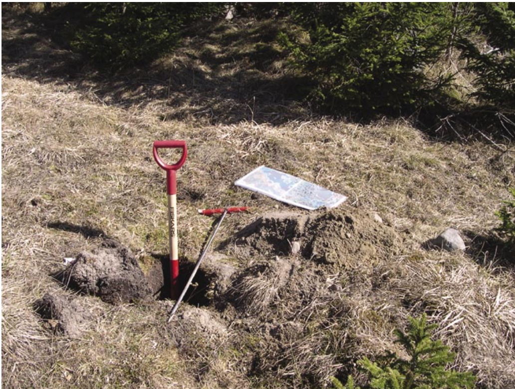
Figure 3-23. The equipment used during mapping of Quaternary deposits. Orientation was made using a hand held GPS and high-resolution IR photos. The geological observations were made in spade dug holes or, more frequently, using a hand held probe.
